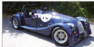
2008. Roadster Lightweight class B race car. Bare chassis rebuild by us with great attention to weight saving to full class B specification in Aero Racing Morgan Challenge Race Series. Including 4 wheel disc brakes vented at the front, 7x15" Image wheels with 225/50R15 Yokohama tyres, modified 3 litre Ford V6, with bespoke ECU, race cams, and big bore manifolds giving circa 280BHP at 7000RPM. She wants for nothing and is ready to race. £39,850
