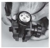
(3) Attach the retainer halves to the cylinder valve.
