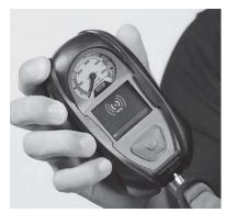
(1) Press and hold BOTH green RESET buttons at the same time until the RFID symbol appears.
