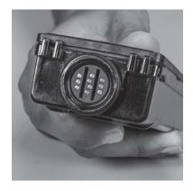
Install the alkaline battery module in the power module:
