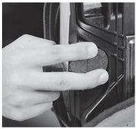
(3) Place the ID Tag over the RFID reader on the power module. The RFID reader is located on the SCBA backplate on the user's right side.
