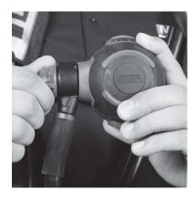
Check the regulator's bypass operation.
