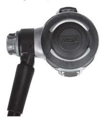
The mask mounted G1 Regulator is a pressure-demand regulator, which maintains a positive pressure in the facepiece while the SCBA is in use. The positive pressure regulator reduces the pressure coming from the pressure reducer further to provide breathable air to the user.
