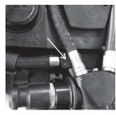
(1) Inspect the elbow connection to the G1 First Stage Regulator as well as the hose connection to the elbow. Ensure that the hose is properly secured.
