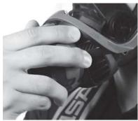
(2) Check proper engagement by pulling on the regulator to ensure that the regulator is securely attached to facepiece.
