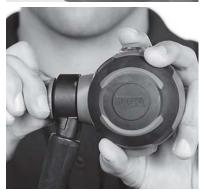
(4) Open the regulator bypass or press the purge button (if equipped) to release system pressure. Close the bypass.
