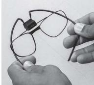
(2) Squeeze in on the wire frame of the spectacle kit at the large bends about 2" from the ends.
