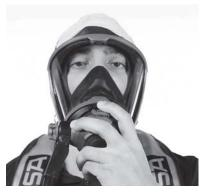
(1) Grasp the regulator and insert it into the facepiece by pushing inward.
