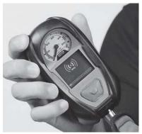
(2) When the battery icon is displayed on the screen, press the ALARM button and RFID symbol will appear.
