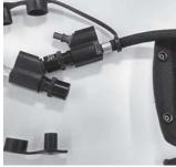
(4) Ensure that the Quick-Connect fittings operate properly and are secured.
