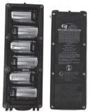
(3) Remove the alkaline battery housing lid.
