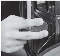
(2) Place the ID Tag over the RFID reader on the power module. The RFID reader is located on the SCBA backplate on the user's right side.
