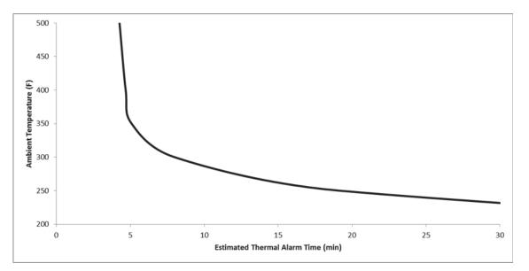
**NOTE**: This chart was generated from data obtained in a laboratory setting and is for reference only. Conditions are highly variable in an actual use scenario. Users of the control module with the thermal alarm option should develop procedures for the use of this feature.
