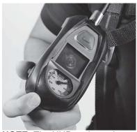
(5) When the pressure falls below 200 psi, turn the control module off by depressing the reset button (green) two times within approximately one second.
