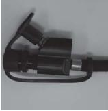
(2) Inspect the dust cover. Ensure that the cover is securely attached to the male and female quick-connect fittings.
