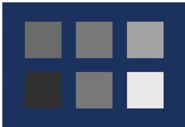
Fig. 4. Two triads with the same difference in differences \Delta d = 12.5 in L^* units. (Upper) L^* = 45, 50, 67.5 , respectively. (Bottom) L^* = 20, 50, 92.5 , respectively.
