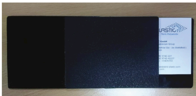
Above: A moulded plaque in an Akro-Plastic laser-transparent compound photographed with a normal camera (left) and with an infrared camera (right)
