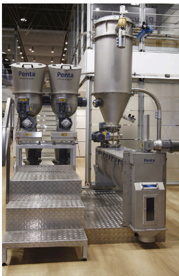
Penta's HurryCon provides smooth and gentle conveying of highly-filled blends in continuous operation
