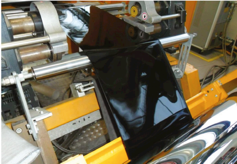
Above: Production of electrically conductive polymer sheet in the Aimplas development lab
