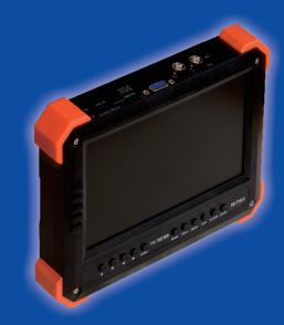
TVI3.0/AHD3.0/CVI2.0/CVBS/ HDMI/VGA INPUT 18650 Li-ion Battery
