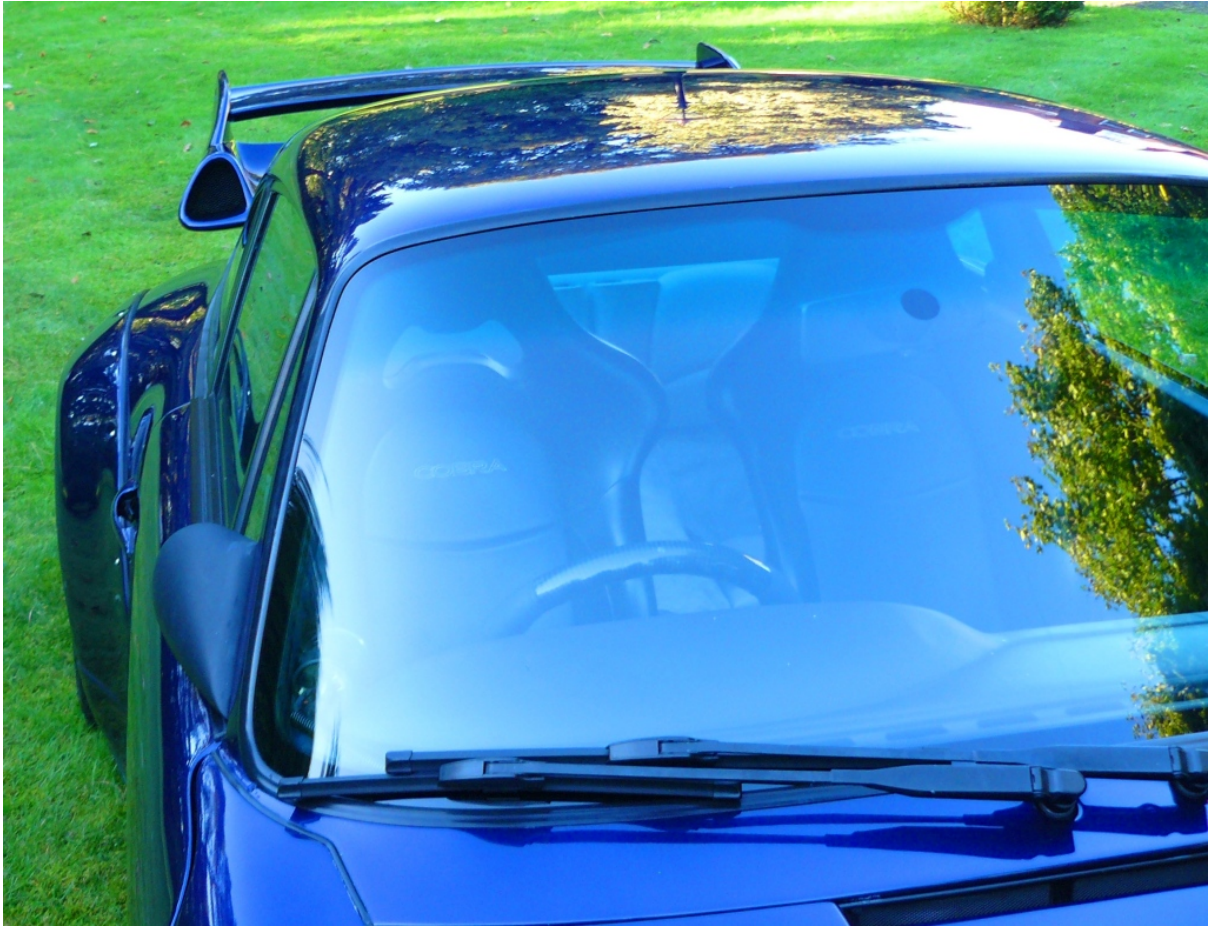
Detail of gutterless roof.
