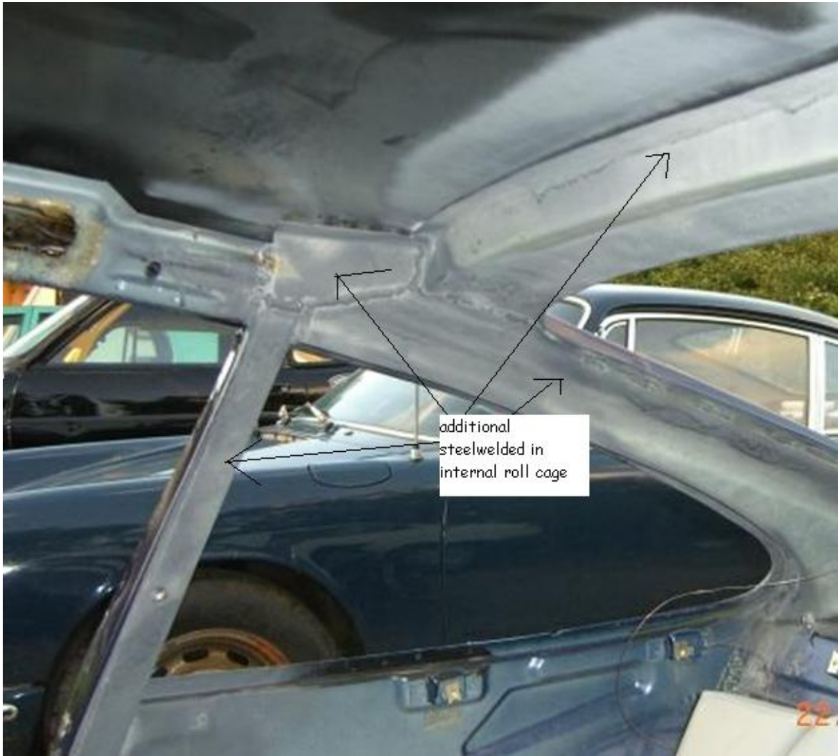
Internal strengthening carried out.
