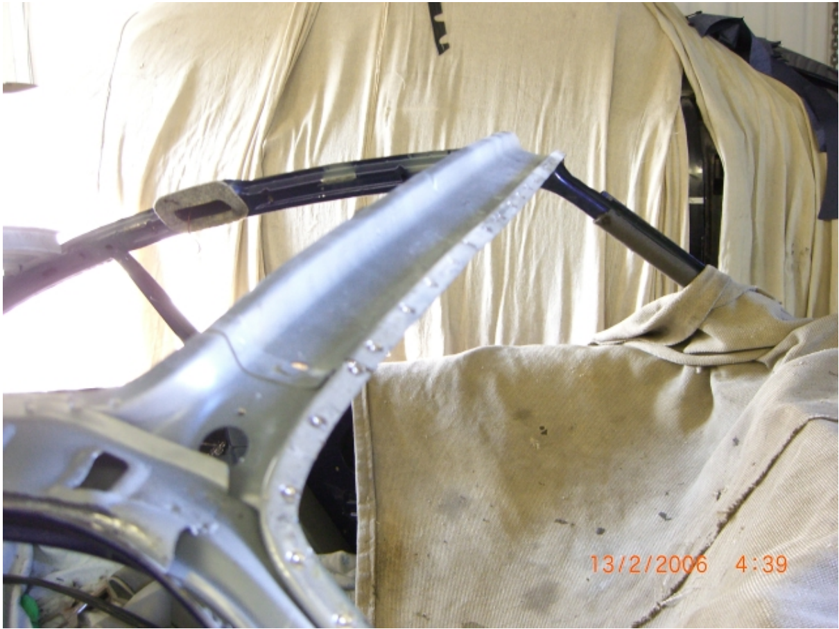
Front internal strengthening at top of window frame.
