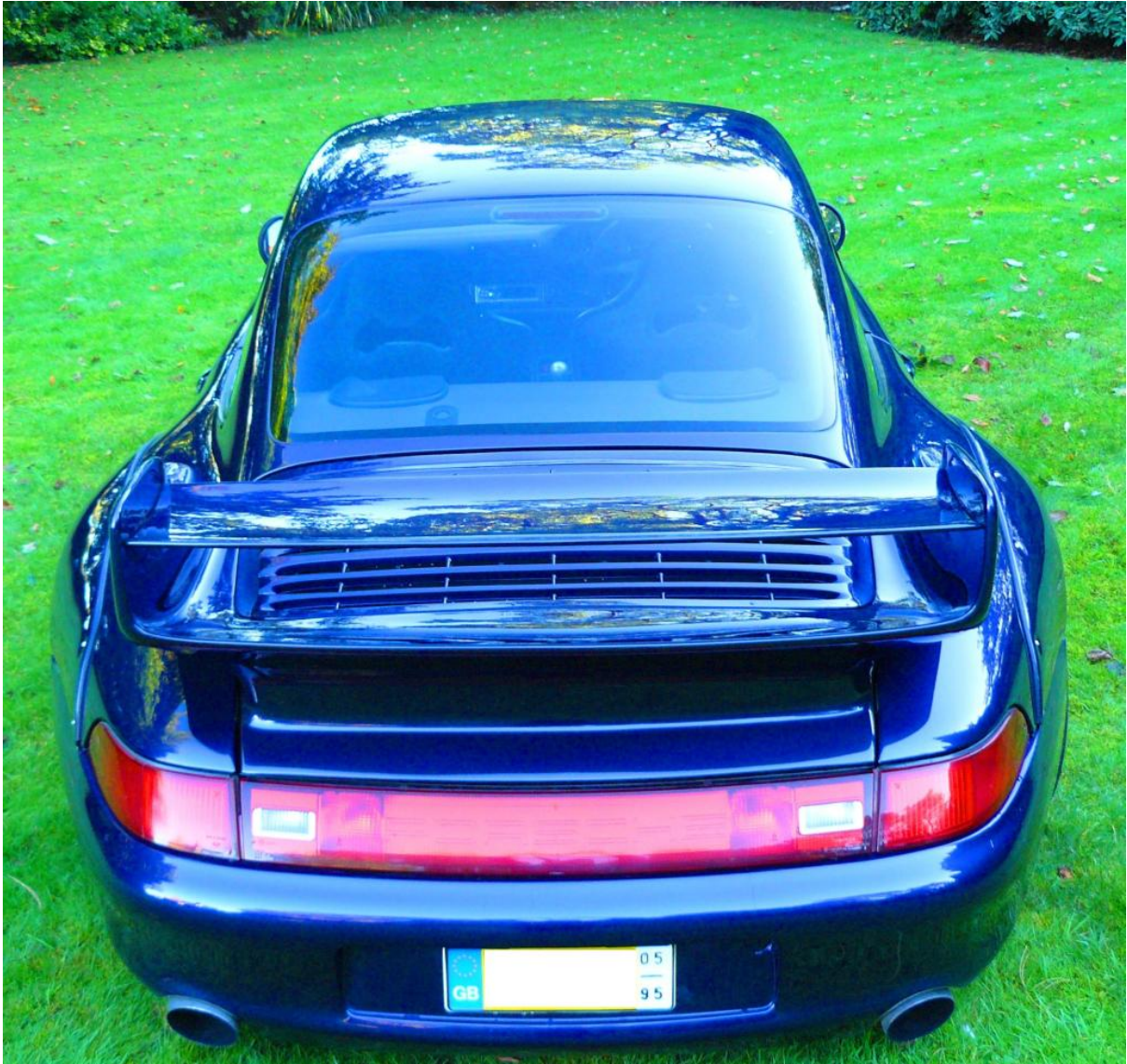
Detail of flush DP Merkalon rear screen and gutterless roof.
