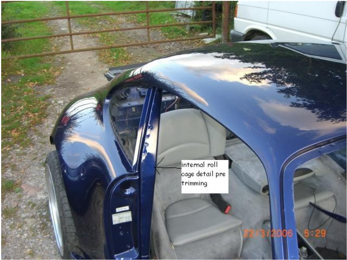
Detail of internal strengthening painted and gutterless.
