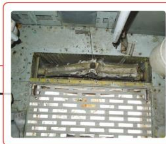
Superheated engine air flowing through a perforated pipe in the vent box under the jump seat—intended to help warm the crew cabin—caused the cushions to smolder and ignite.
