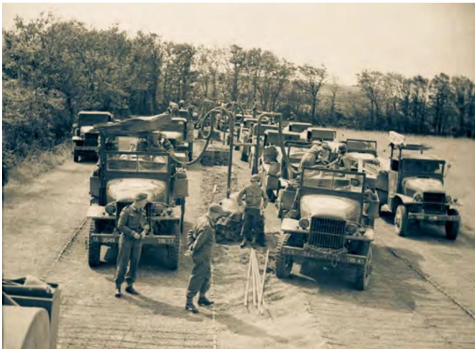
Red Ball Express trucks taking on fuel. The fuel point is reinforced by metal standings for better traction. SGT. HARRISON NO.5 ARMY FILM AND PHOTOGRAPHIC UNIT / WIKICOMMONS
