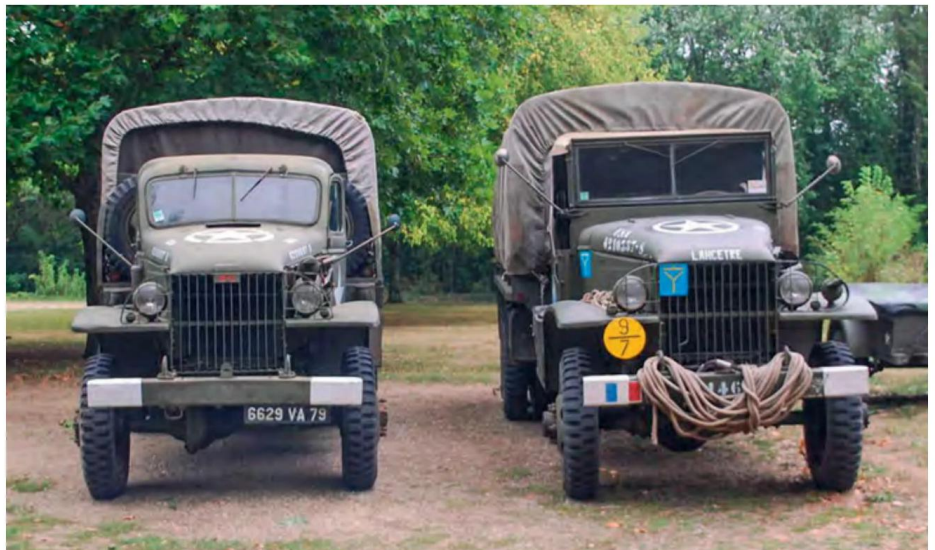
Bringing the Red Ball Express back to life, Alain's CCKW 352 alongside an open-topped CCKW 353. Interesting to see the different heights of the vehicles
