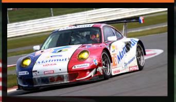
Powering the 911 GT3 RSR is a particularly efficient six-cylinder boxer engine with a four-litre capacity. With a mandatory airrestrictor, it generates 460 hp (338 kW) and drives the 310 millimetre wide rear wheels. The diameter of the front wheels has increased by 30 mm to measure 680 millimetres. The Porsche sequential six-speed gearbox is operated via paddle shifts on the steering wheel.
