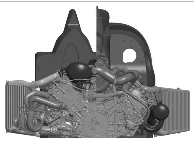
Side-by-side comparison of the engine bays of the R15 V10 TDI (left) and the R18 V6 TDI (right)
