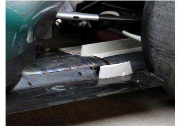
A further iteration of the exhaust blown floor, as seen on the Mercedes, showing the attachments to channel airflow through the diffuser
