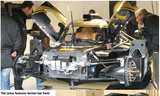
The Lotus features torsion bar front suspension, not seen on an LMP2 design since the Porsche RS Spyder
