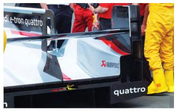
The Audi's Le Mans specification rear end features a lower rear wing. The double rear wing end plates are directly inspired by the TS030
