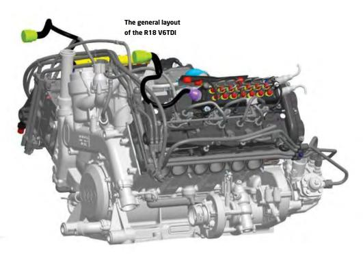
designed around several key areas: the bearing load through the RPM range and load spectrum (ignition pressure and inertial forces); torsional and bending stiffness; free moments of the first and second order; vibration sensitivity and lightweightness.
