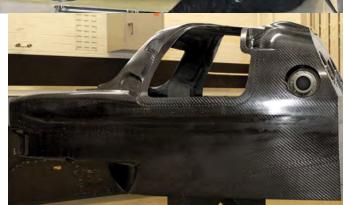
Bodywork consists of carbon sandwich composite panels, with quick release nose, rear diffuser, wheel arches, rear end and rear wing
