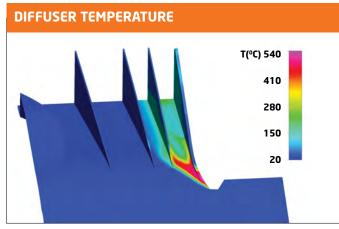
Top: the vortex from the rear wheel of the Pilbeam with an unblown floor can be seen to reduce the overall efficiency of the diffuser Bottom: the blown version of the floor, showing the temperature of the exhaust gases into the diffuser (both images from Thijs van Rees' thesis)
