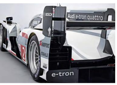
Audi is believed to be playing with the air pressure behind the rear wheel to reduce drag (see separate feature).
