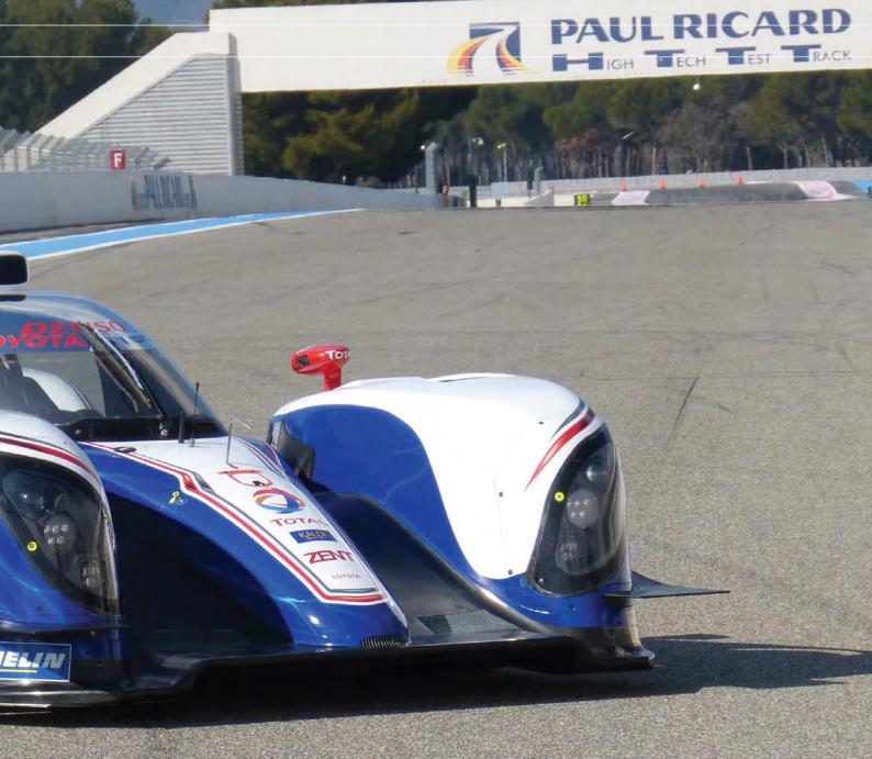
of 2012. The tub used last year was designed to evaluate both front and rear hybrid systems, and the team raced with the compromised chassis. Now that it has settled on a rear-only solution, the tub has changed to reflect that, leading to a new, tightly controlled aero package. The new nose is lower, and the change means that the team will have to re-crash test the tub ahead of its first race.
