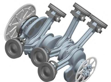
The obliquely divided steel connecting rod is manufactured with an optimised profile and further refined with regard to stiffness, optimum dynamic bearing stability and minimum weight by FEM calculation
