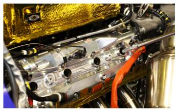
Toyota's V8 engine does not feature direct injection, but it is thought that the 2014 specification unit will
