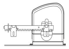
the cogwheel, previously unlocked, as in Fig. 5. Fix the element to the gate, in the way you wish, by applying to it the other elements of rack necessary, ensure that all be united and aligned. Locate the desired position and fix end-run device (F) on rack as indicated in the previous Fig. 2, those with grains included. Close the release lever and perform the necessary electrical connections.
