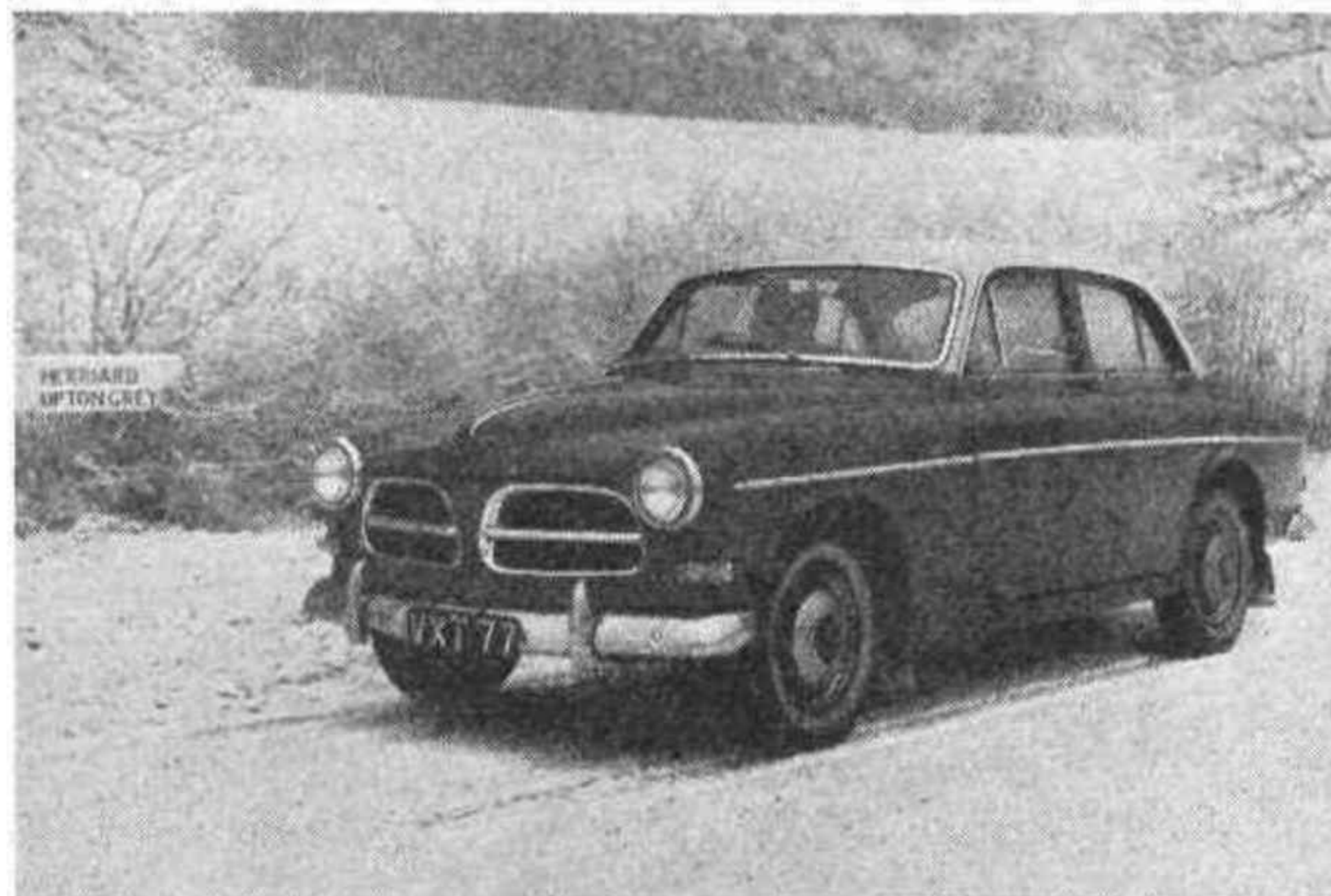
REMARKABLE FOR A 1.6-LITRE SALOON, the Volvo 122S will exceed 50 m.p.h. in second gear, show a speedometer reading of more than 80 m.p.h. in third gear, and has a maximum in top of nearly 95 m.p.h., with acceleration and controllability in keeping!
