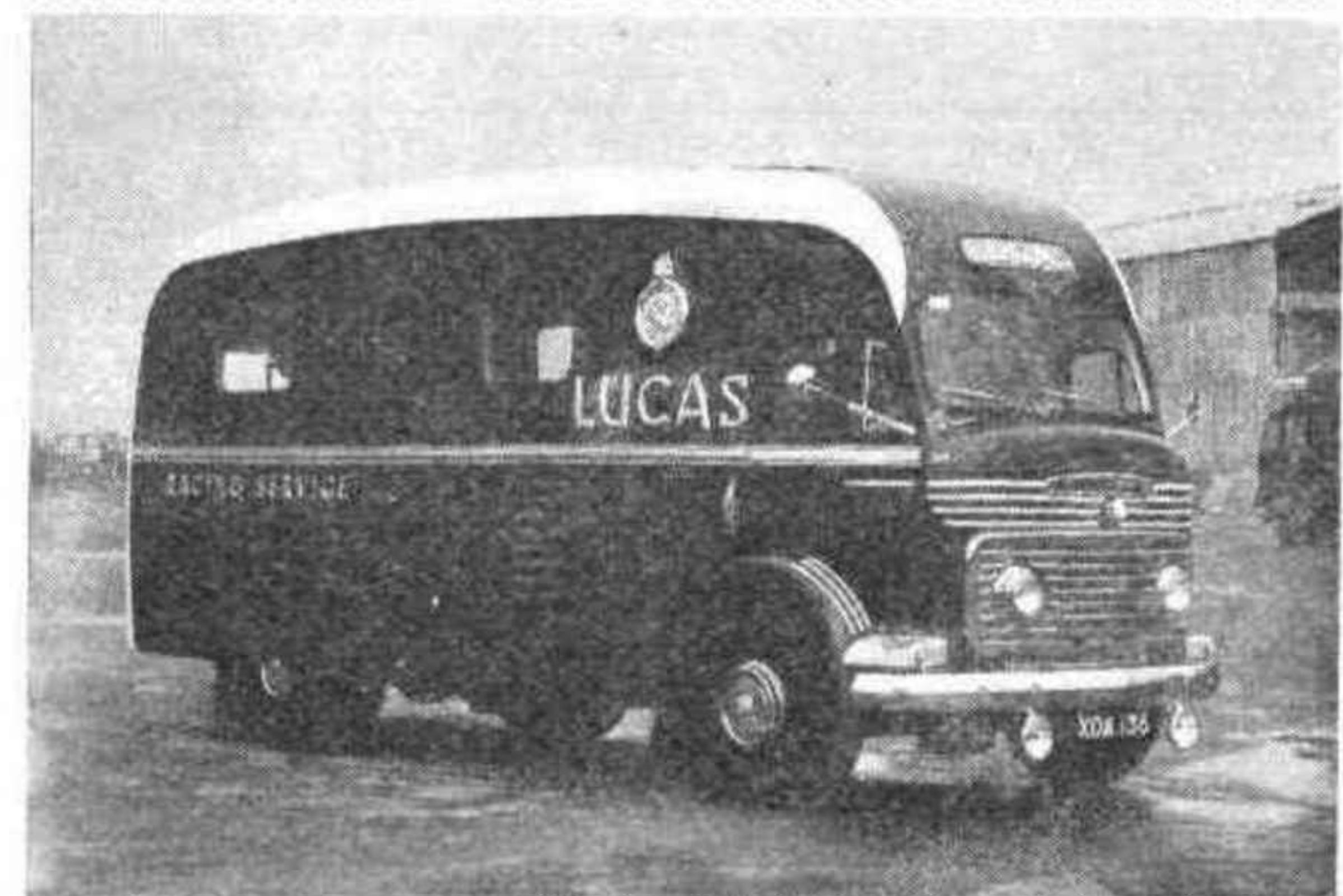
AID FOR COMPETITORS.—Starting with the Monte Carlo Rally, Joseph Lucas, Ltd., will operate this new Commer TS3 Racing Service van. The body was built by the Lucas Transport Department to the Racing Department's specification and equipment includes lathe, drilling machine, magneto test bed, bench grinder, etc. Power for the workshop is provided by a 5KVA petrol generating set.
