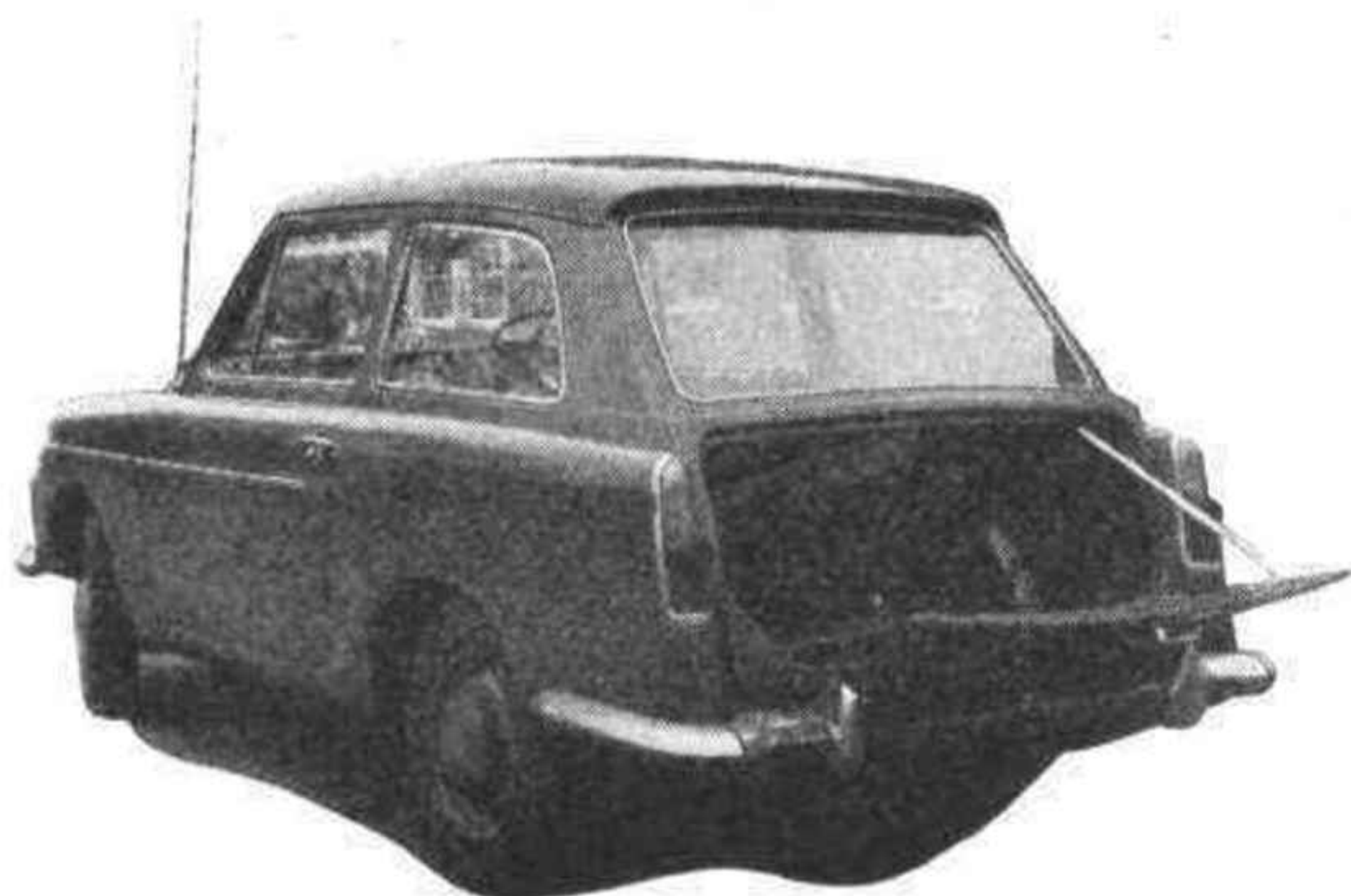
LUGGAGE CARRYING ARRANGEMENTS of the new Austin A40. This picture shows how the fixed rear window restricts the loading aperture. The door is not intended to be used as a luggage platform and the wheel arches and floor-mounted spare wheel obstruct the luggage compartment. The back door is lockable.
