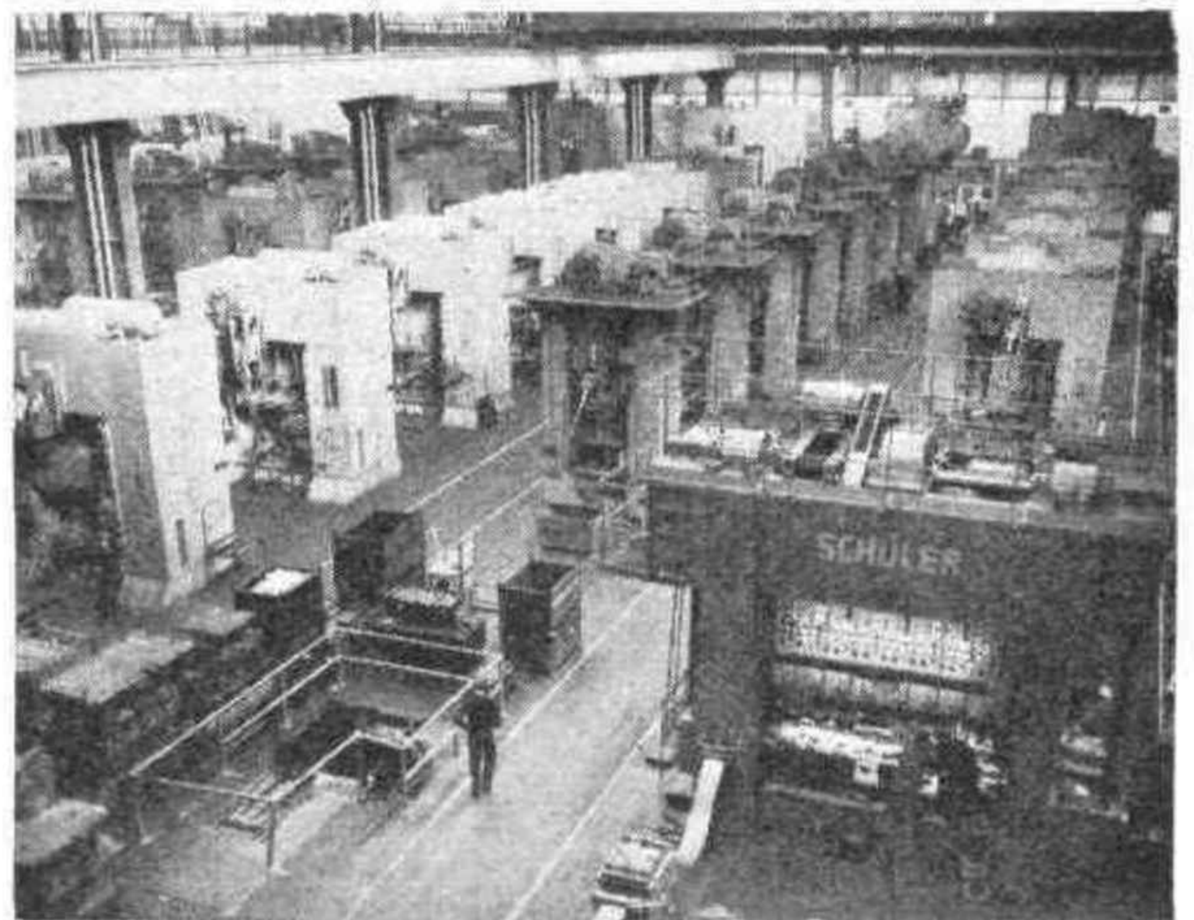
The imposing new Press shop at Vauxhall Motors, Luton, factory with one of their new German Schuler small-parts automatic transfer presses in the right foreground.
