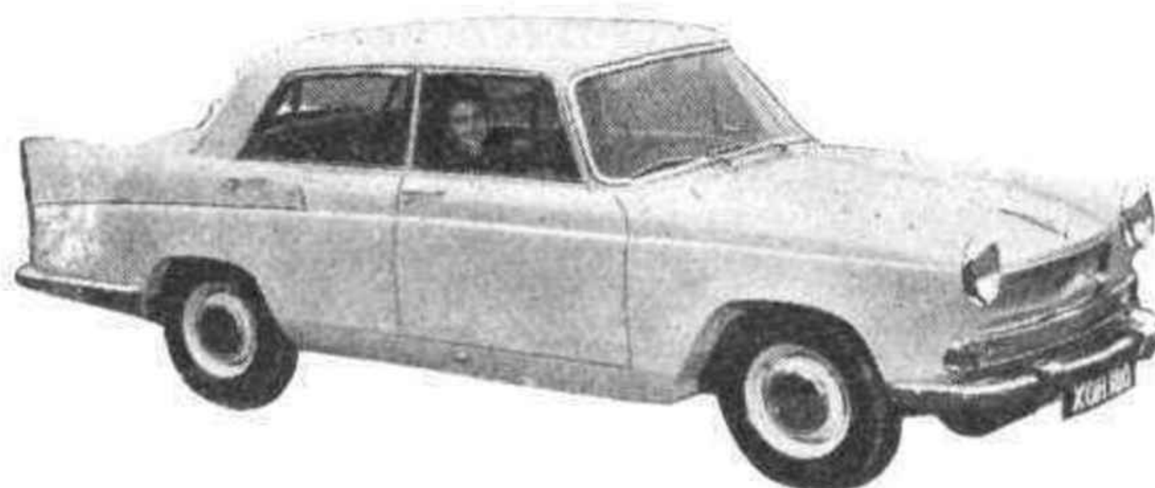
A NEW AUSTIN. —This Austin A55 is the third of the new Pinin Farina-styled B.M.C. cars. The engine has modified manifolding, resulting in an output of 53 b.h.p. at 4,250 r.p.m. The car is longer, wider and about one hundredweight heavier than its predecessor and costs £848 17s. in standard form.
