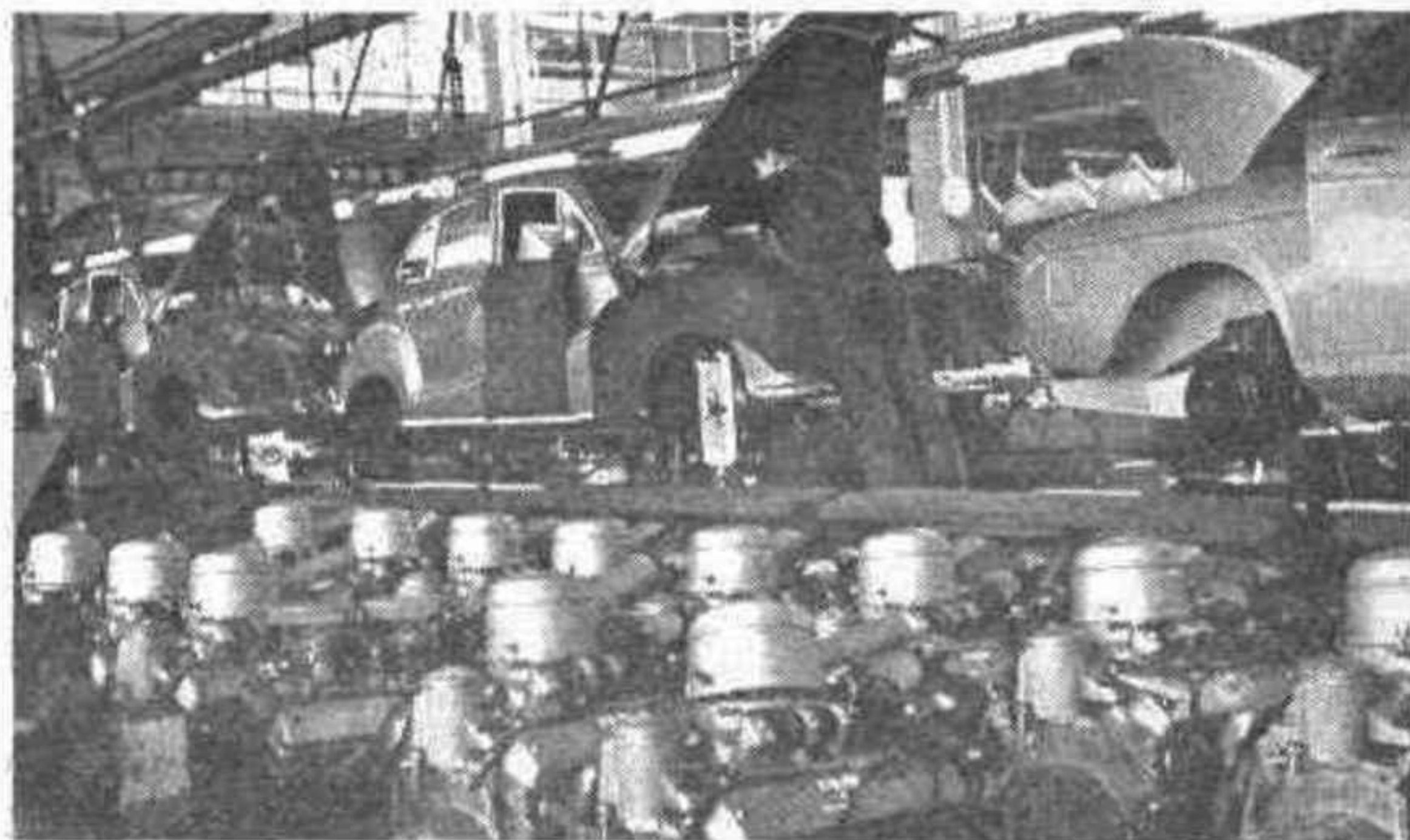
B.M.W. ASSEMBLY-LINE. —The neon-lit, raised assembly line where B.M.W. cars near completion, with 2.6 and 3.2-litre V8 power units awaiting their turn to go out into the world and work.
