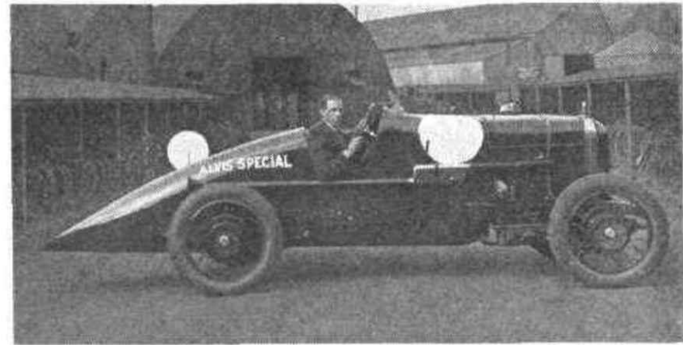
A RARE PICTURE of the works 12/50 Alvis which Sutton drove in the 1926 J.C.C. 200-Mile Race at Brooklands, backing up Harvey and Cottenham in the front-drive straight-eight Alvis cars. It had dry-sump lubrication and this, and the slightly-cowled radiator and streamlined oil tank adjacent to the rear side of the chassis, were reminiscent of the 1923 200-Mile Race winner and may have come from that car.
