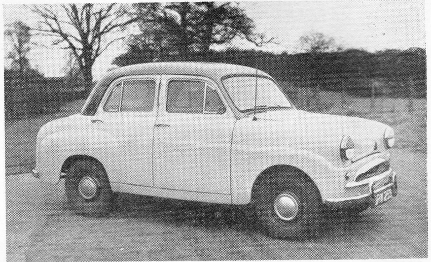
NEW "TEN" FROM CANLEY: (Above) The latest Standard model, with 948 c.c. o.h.v. four-cylinder engine, which will retail at £409, plus P.T., when available on home markets.
