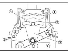
Remove the two screws and remove the throttle lever assembly. Position the throttle lever assembly so that it faces downward and secure it with the two screws.
