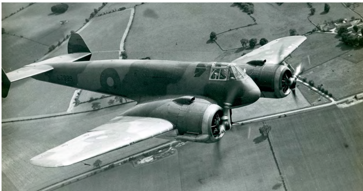
RIGHT The first Gloster F.9/37 prototype, L7999, undertaking an air-to-air photographic sortie. Test pilot Michael Daunt is believed to be at the controls.
