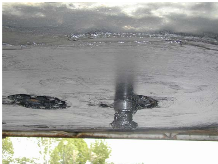
Figure 4.27 Kingpin on trailer underside for fifth wheel coupling.
