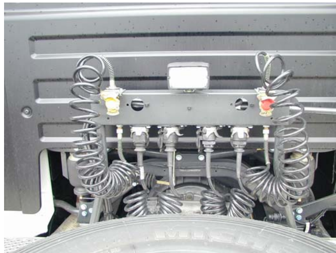
Figure 4.25 Trailer connection for automatic coupling (required)
