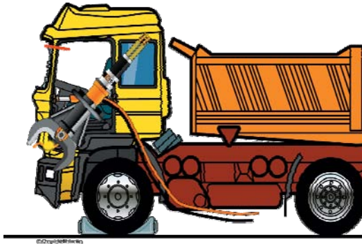
Figure 4.32 Cut any strengthening cross members if they can be easily accessed. Remember some materials used in modern construction may be difficult to cut with conventional cutting tools.
