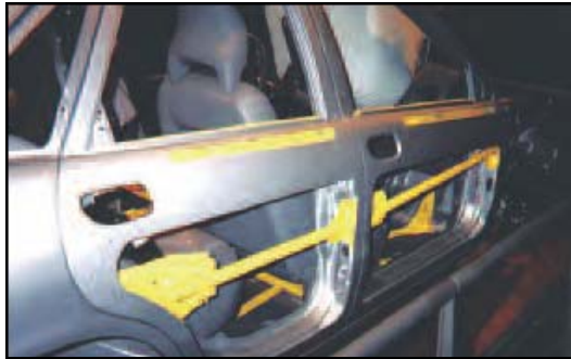
Figure 4.6 Side impact bars
