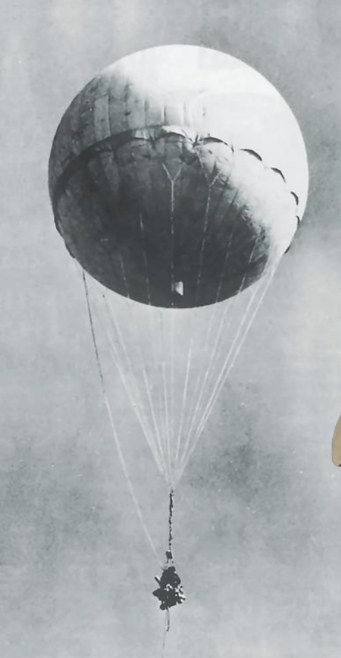
An intact specimen found near Alturas, California, was later reinflated for study at Moffett Air Base (left). The balloons carried ballast and bombs timed to go off at the end of their journey (far right). Opposite, left: men at Moffett restrain the inflated balloon.
