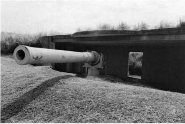
The two Momi guns are 6-inch MkVIIIs on MkII central pivot mountings. This was a combination introduced into service in 1898 and the markings on the guns indicate that they were manufactured at the turn of the century by Vickers, Son and
