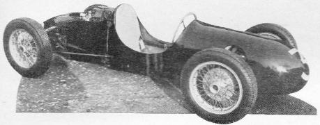
LATEST "500": Three views of the new Petty-Norton, built by Ray Petty, and first raced by A. V. Cowley at Brands Hatch on Boxing Day. The design features a de Dion-type rear axle (below, left) with transverse leaf spring; front springing (below, right) is by wishbone links and top rocker arms to hydraulic suspension units mounted within the ladder-type tubular frame.
