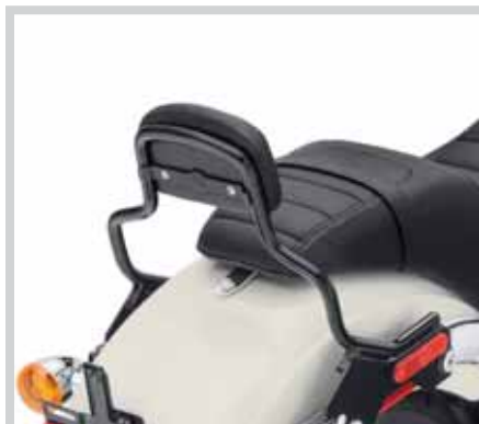
A. SHORT HOLDFAST SISSY BAR UPRIGHT – GLOSS BLACK (LOW RIDER MODEL SHOWN)
