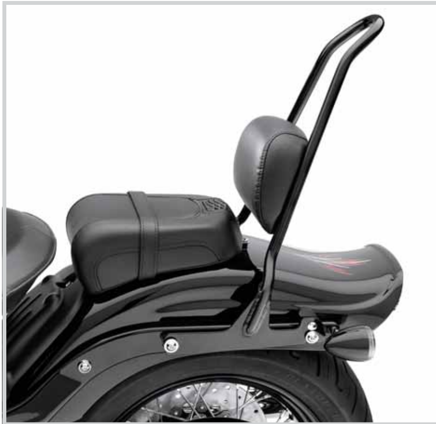
A. ONE-PIECE H-D DETACHABLES TALL SISSY BAR UPRIGHT – GLOSS BLACK (SHOWN WITH PASSENGER BACKREST PAD)
