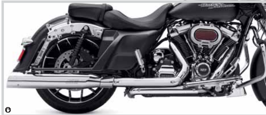
A. SCREAMIN' EAGLE HIGH-FLOW EXHAUST SYSTEM WITH STREET CANNON MUFFLERS CHROME WITH CHROME MUFFLERS
