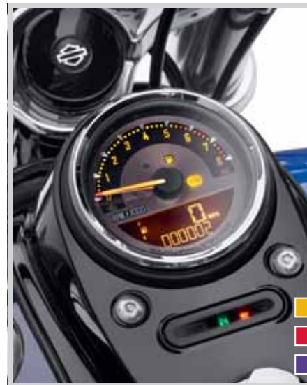
B. DIGITAL SPEEDOMETER/ANALOG TACHOMETER – 4" SPUN ALUMINUM DIAL
