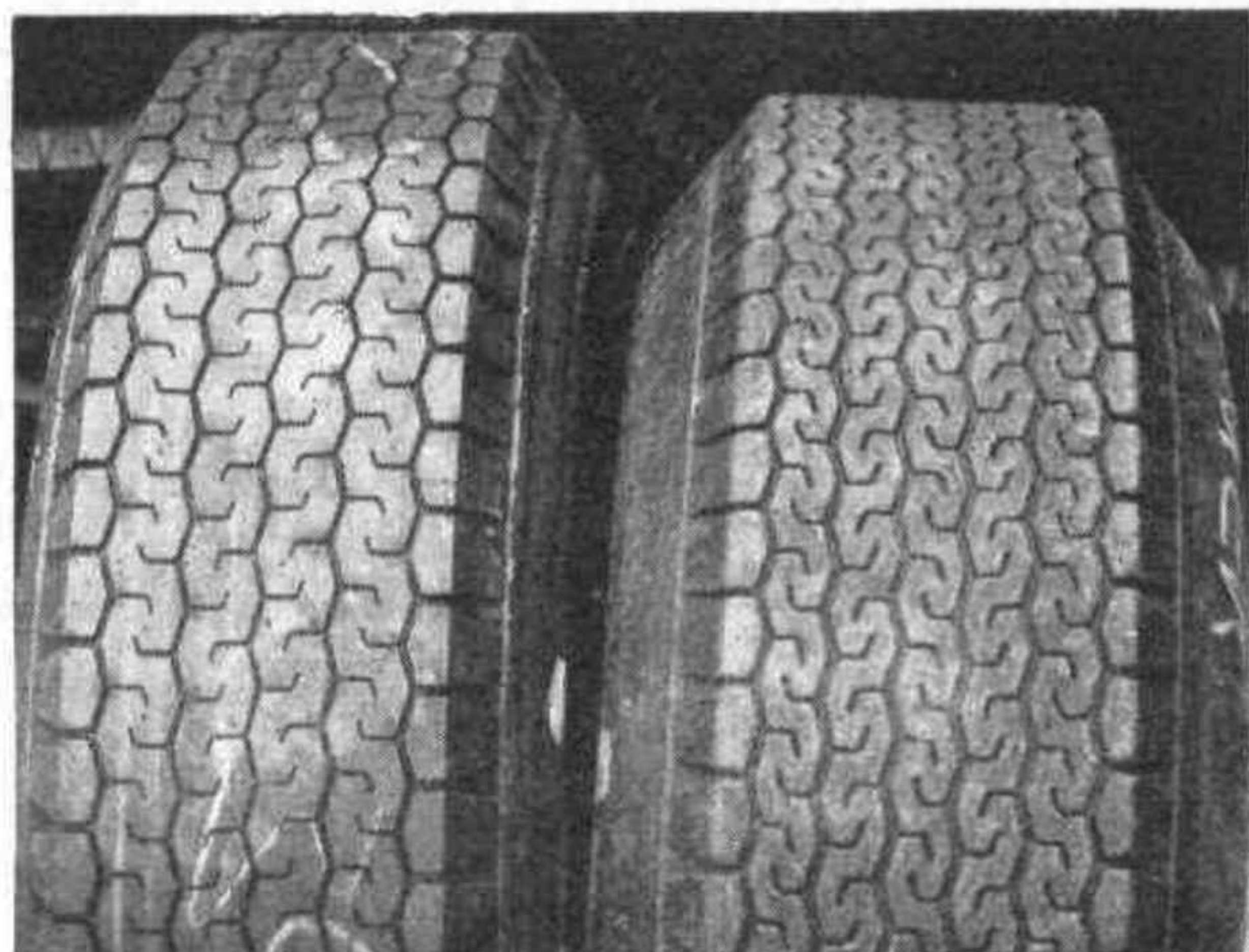
NEW DUNLOP R7.—The New tread pattern for the Dunlop R7 is seen on the left with the original R7 on the right. The new pattern holds less air in the tread and has a lot more rubber in contact with the road.
