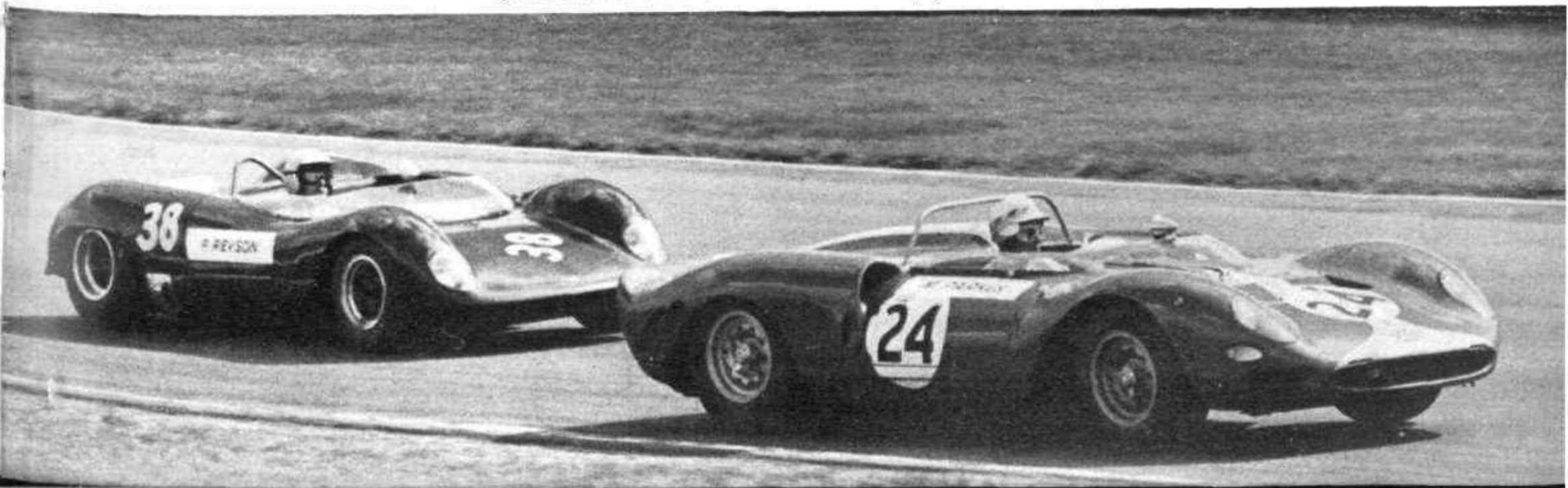
▼ DUAL PURPOSE. —Mike Parkes drove a 375P/2 Ferrari, changed from a Prototype to a sports car by fitting a small windscreen and a crash bar in place of the Le Mans "wing" behind the driver's head. It was very outclassed among the "Hot Rods" and here is followed by Revson's immaculate Brabham BT8 with 4-cylinder Climax engine.
