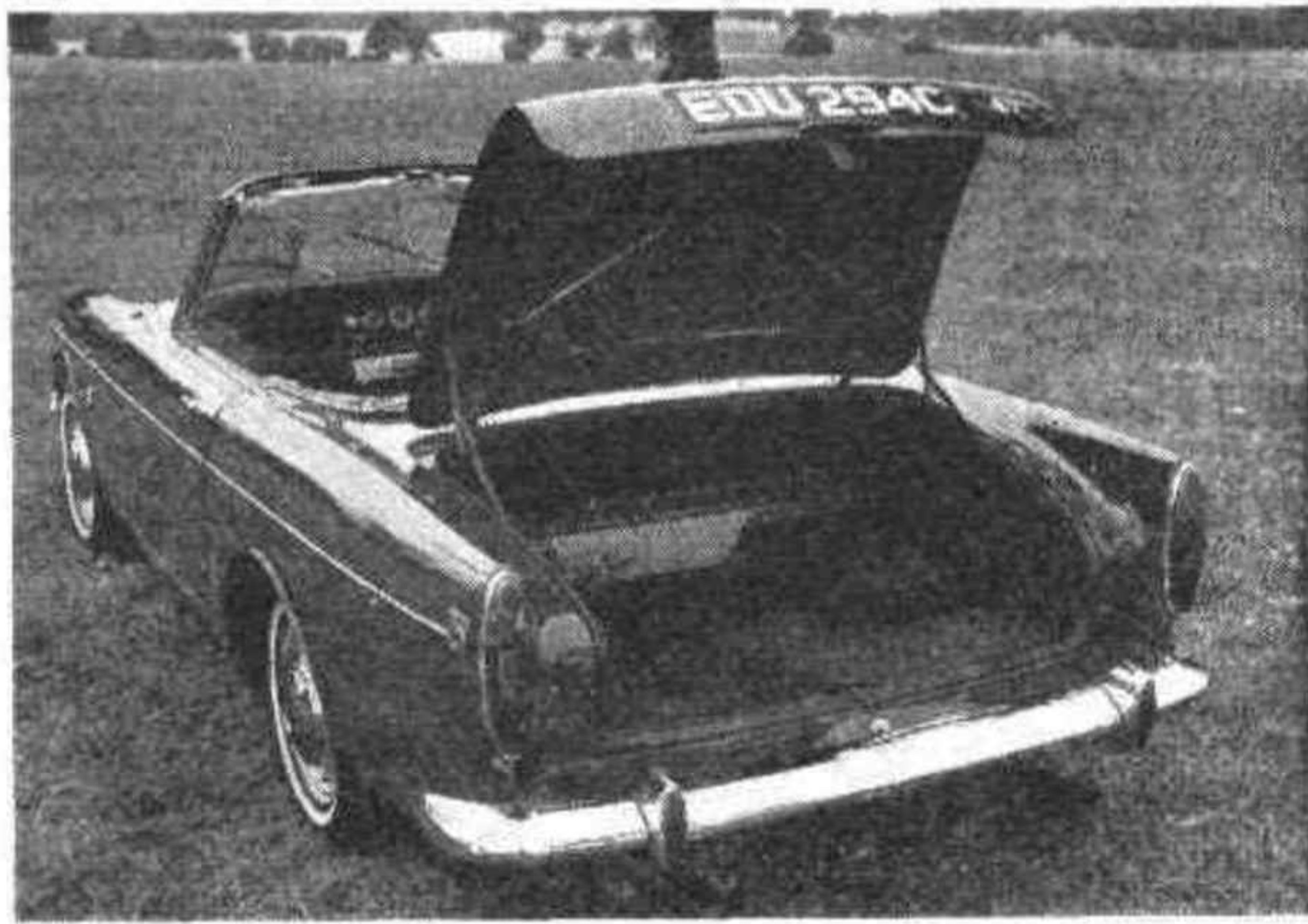
TIGER DETAILS. —Left view shows the well-appointed interior, comfortable seats, central gear-lever and acceptable facia of the car, that on the right the size of the luggage boot, with spare wheel and battery stowed under the floor.
