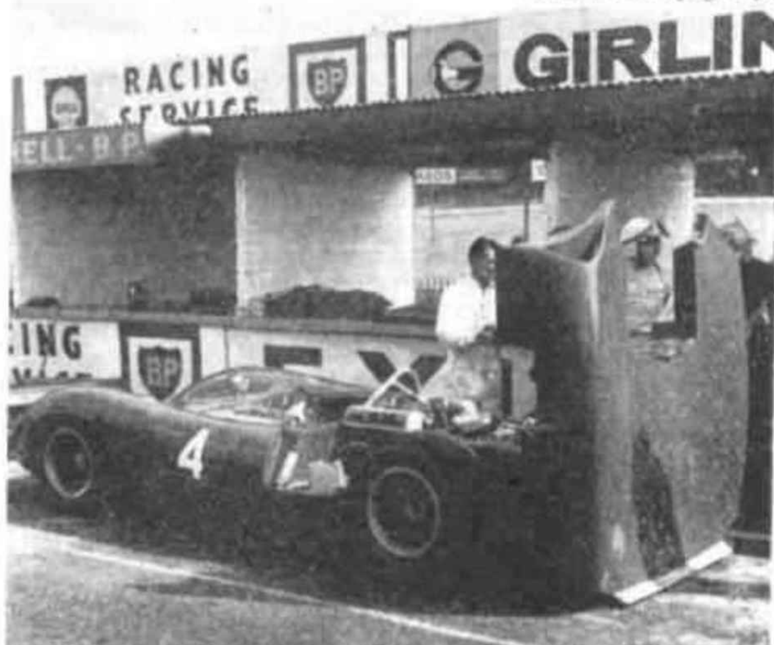
ONE PIECE. —On the Lola 70 the complete tail hinge, up to allow access to the engine compartment, and is easily detachable if serious work has to be done. This is the Guard's Trophy-winning car of John Surtees.
