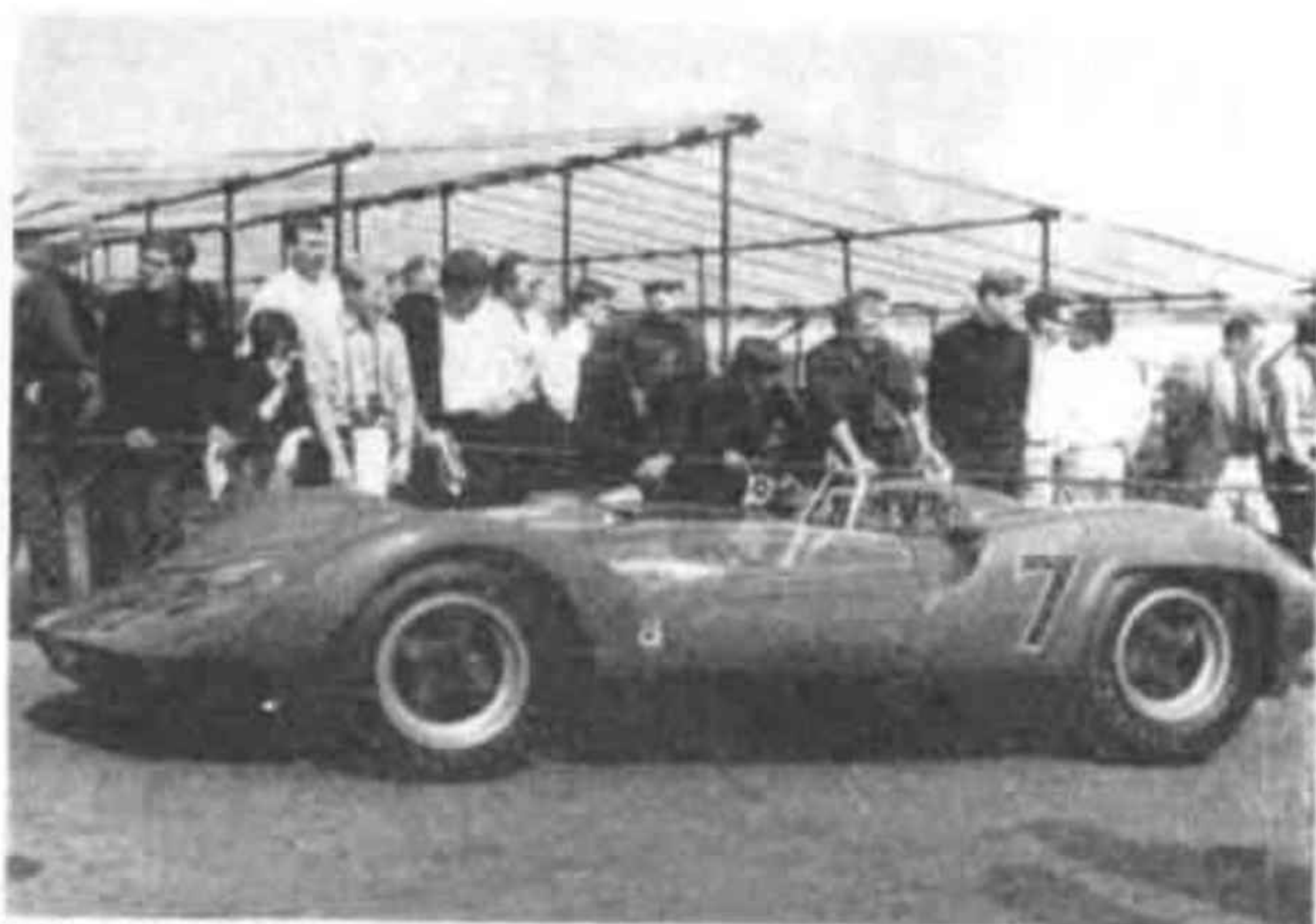
TWO-SEATER RACER. —The McLaren-Elva-Oldsmobile of Bruce McLaren in the paddock at Brands Hatch. The lower part of the body between the wheels is formed, on each side, by a fibre glass covered aluminium fuel tank.
