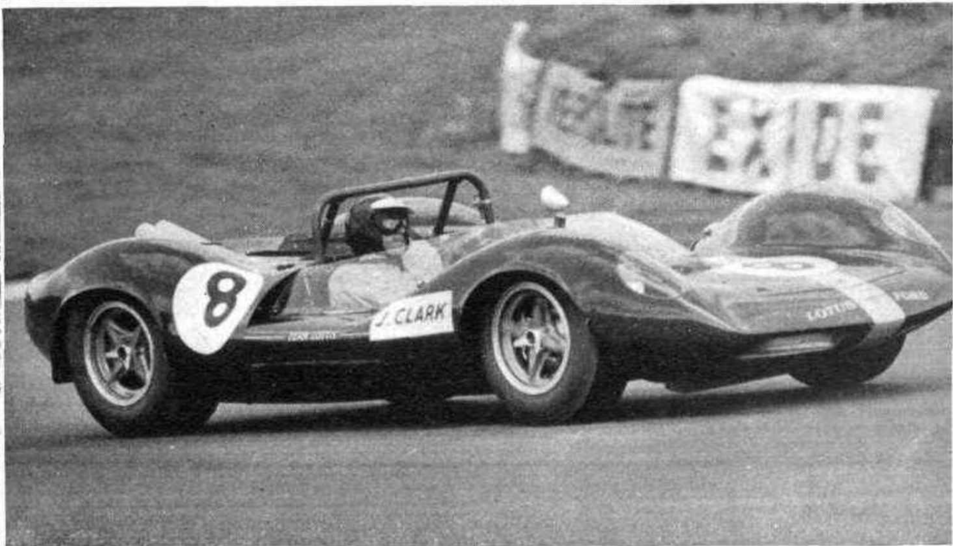
▲ TOO NEW. —Jim Clark drove the brand new Lotus 40, making its first appearance in the Guards Trophy. It has a 5.7-litre Ford V8 engine, Climax-type exhaust system, and 15-in. wheels among other new features. Lack of practice prevented it being sorted out properly.
