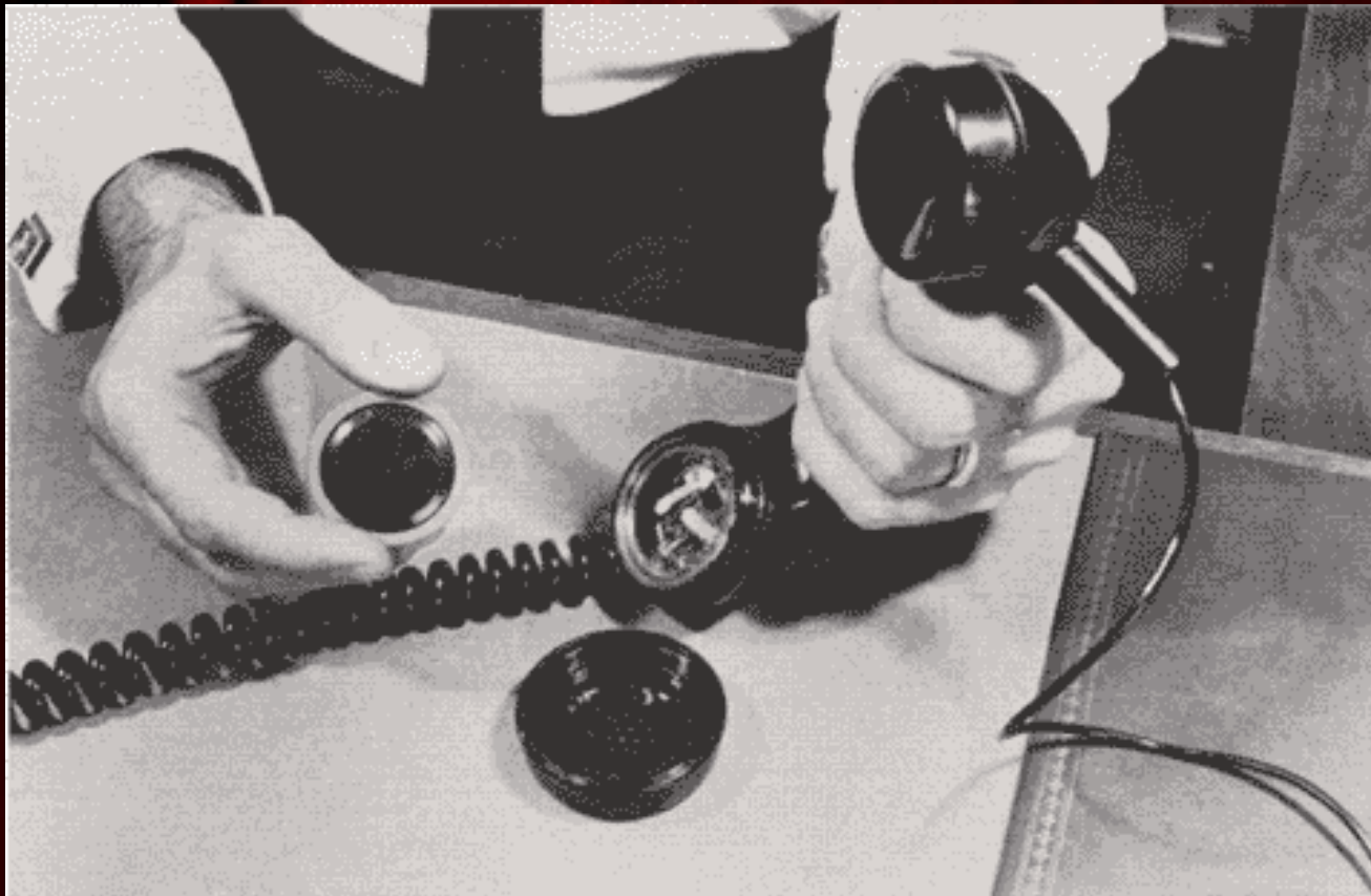
An expert holds a small microphone that can be hidden behind a telephone mouthpiece.
