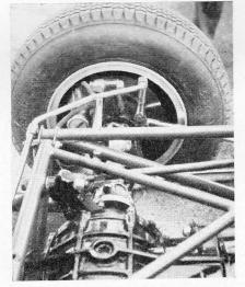
THE REAR end of the F.J. car showing the outboard-mounted disc brakes and anti-roll bar mounting points.
