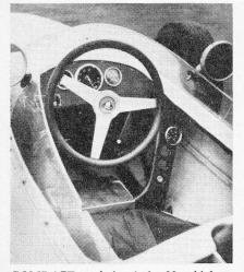
COMPACT cockpit of the 22 which retains reclining seating position but now has "left-hand" gear lever.
