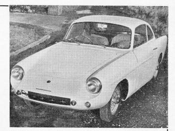
WITH MODIFIED FORD 109E ENGINE, GIVING 70 B.H.P. DISC BRAKES ON THE FRONT 13" WIRE WHEELS. WOOD RIM STEERING WHEEL. COMPREHENSIVE INSURANCE ONLY £28 FULL INSTRUMENTATION. ASSEMBLY CAN BE COMPLETED IN 24 HRS. USING ONLY HAND TOOLS
