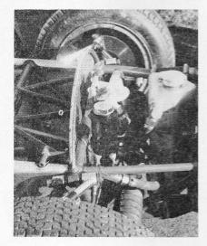
ABOVE: The oil tank for the 1,100 c.c. F.J. engine which is mounted right behind the radiator. Note the outboard-mounted Girling discs.
