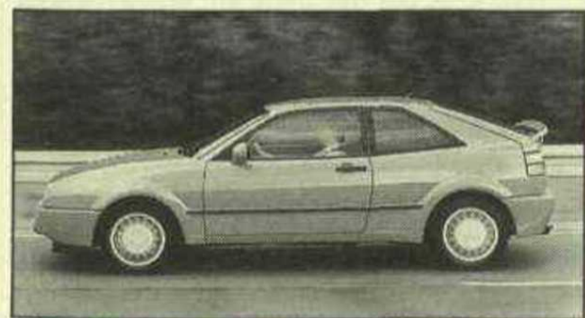
Speed triggers a 50mm rear spoiler extension.
