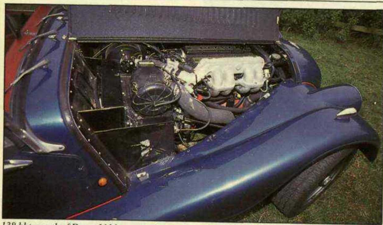
138 bhp-worth of Rover M16 squeezes into heavily-louvréd tapering nose.
