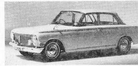
THE NEW VAUXHALL Cresta (above) and Velox announced this week combine new looks and interior treatment with a well-proved, highly developed technical specification. The 113 b.h.p. 2.6-litre engine has a compression ratio of 8.5:1, and Hydra-matic fully automatic transmission is an alternative to an all-synchromesh three-speed gearbox, which has overdrive on top and second as an extra.
