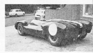
REAR VIEW of the interesting new Cooper Monaco, the Type 61, which has a 4-cylinder, 2.7-litre Coventry Climax engine.
