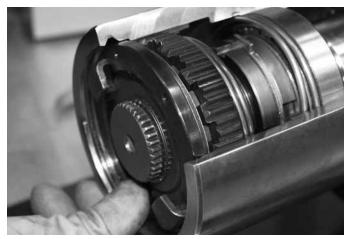
12. Test for proper operation of the cam spacer by compressing the spacer into the hub several times. The cam spacer must freely slide in and out of the hub assembly and return fully seated against the retainer plate. If any binding or resistance occurs disassemble all components and check for proper assembly.
