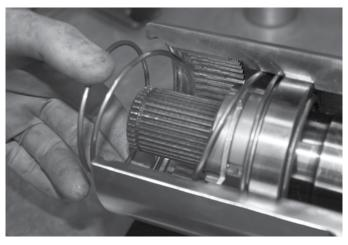
7. Coat the spacer with high pressure grease on all surfaces. Assemble spacer over the outer axle and seat it against the spindle or snap ring. Different spacer heights are available for different hub applications. Verify the Lockout assembly part number and proper application before moving forward.
