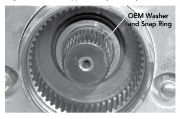
4. Before installing lock-outs inspect the splines inside the hub to verify there are no burrs, rust or any other debris. Thoroughly clean and debur the inner portions of the hub.
