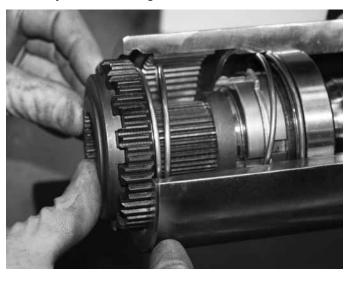
9. While fully compressing the assembly install the axle snap ring if applicable. Assure the snap ring fully seats into the groove on the outer shaft. If no outer snap ring groove exists proceed to the next step in assembly.
