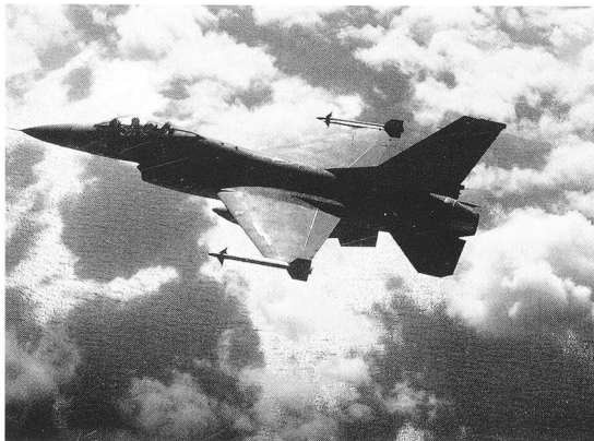
Jax interceptors carry dual AIM-9 Sidewinders for alert scrambles. Birds will soon be fitted with radar-guided AIM-7 Sparrows as well.
