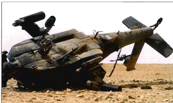
While serving as a QRF for the 3rd ID on 31 March 2003, the crew (CW2 Mike Carman and CW3 Cathy Jarrell) of AH-64D 99-5104 was scrambled on a medevac escort. Moments after lifting off, the aircraft got into brown-out conditions and the main rotor struck the ground, rolling the helicopter onto its back (US Army)
