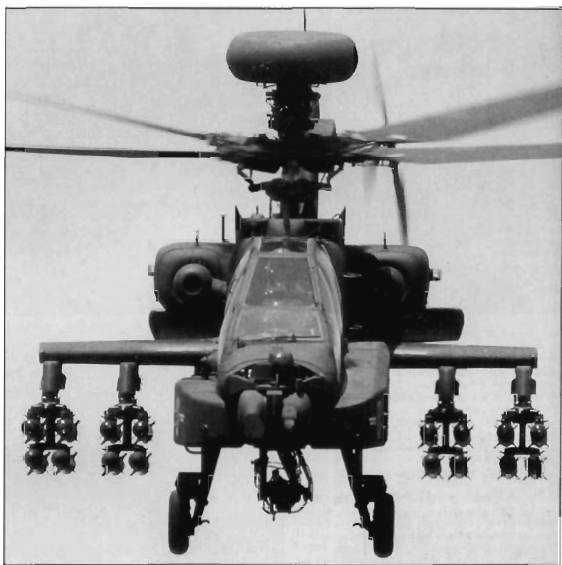
McDonnell Douglas' AH-64D Longbow Apache demonstrator is seen carrying a full weapons load of 16 Hellfire missiles during a press demonstration in the mid-1990s. By 1997 this aircraft was wearing Boeing titling (Ted Carlson)
