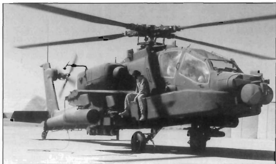
This Lot 7 Apache from the 'Avengers' of A Company has just undergone a phased maintenance inspection and is conducting an engine run-up (CW2 John Rawls)
