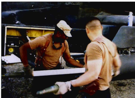
Pilots from B Company load M151 10-lb HE rockets into the outboard M261 launcher. Groundcrews often had their hands full maintaining the unit's hard-worked helicopters, so pilots would gladly assist with the rearming of their aircraft (CW4 Zac Noble)
