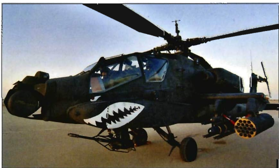
Featuring a newly applied 'sharksmouth', this 4-3 ACR AH-64A carries the now-standard mission load-out of one IR Hellfire and two rocket pods per stub wing (via John Musick)
