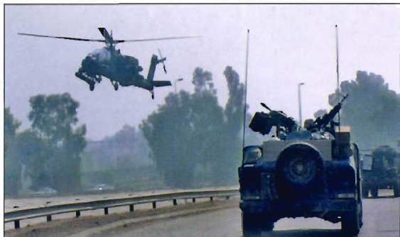
Increasing threats from the Sadr City district of Baghdad warranted increased Apache patrols over the city in support of 1st Cavalry troops sweeping the area in August 2004. Here, a 1-1 AVN AH-64 covers a heavily armed and armoured Humvee fitted with an M240B and MK19 automatic grenade launcher (US Army)
