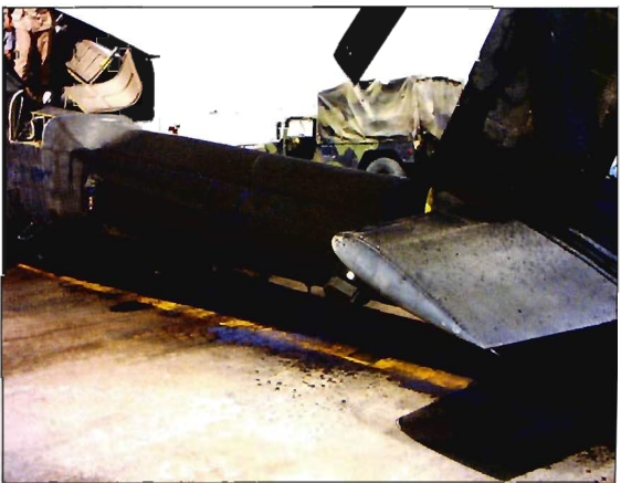
AH-64A 89-0260 from B Company 'Raiders' was photographed soon after landing at Kandahar without any transmission fluid. The contents of the entire transmission fluid reservoir can be seen spread across the helicopter's tailboom (CW4 Zac Noble)
