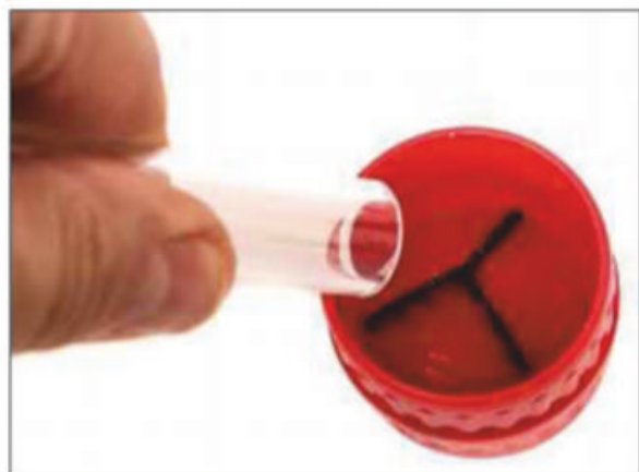
The deburrer's angled blades score the inner and outer edges of the tubing, removing rough edges
