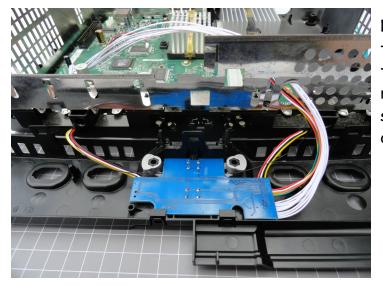
Next insert the XeniumRGB front panel into the faceplate and run the two main cables through the hole as shown in the image. And run the Kynar dimming wire's through the same path as the 4pin cables for each set of ports.
