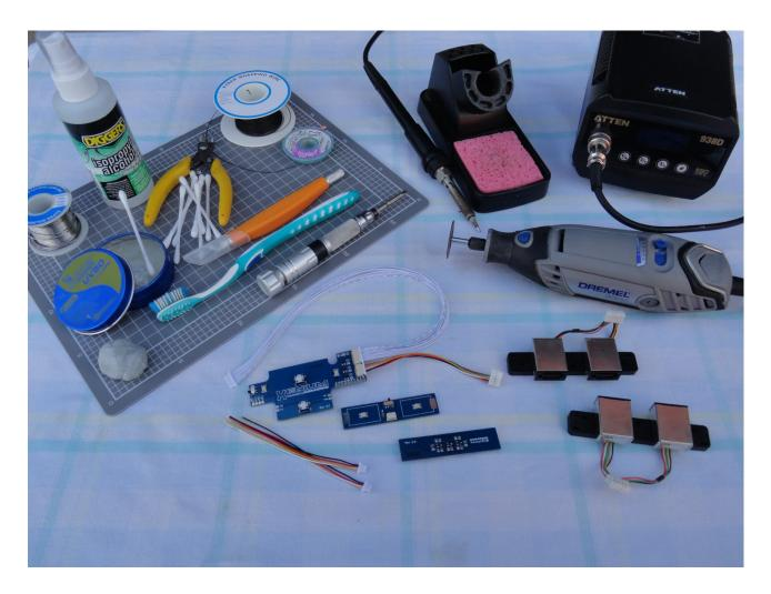
In addition to the usual recommended tools we will need a "Dremel" or similar device to cut the shielding on the back of the controller ports off.
