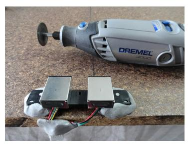
Now we will prepare the controller ports for installation, I was able to mount the ports to my workbench using "Blu-Tack" which gives a good enough hold while you work on it.
