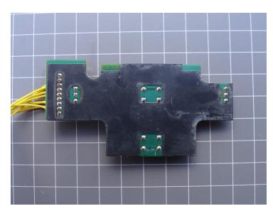
On the Original Xbox front panel there's a layer of insulation. I can see the reasoning behind this as the PCB is hard up against the shielding and overtime the vibrations could wear through the solder mask and a short may occur.
