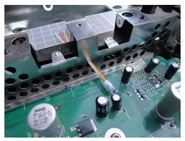
For the full XeniumRGB front panel and controller port install, start by passing the 4pin "DIY" cables through the hole in the shielding as shown in the image.
