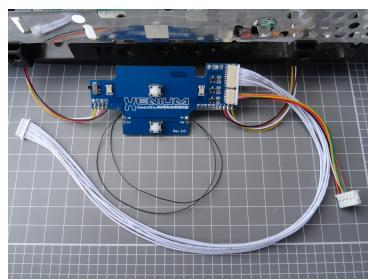
It might get a little tight to work on since the 4pin cables are rather short but after having soldered all the wire's and plugging in the 10pin and 6pin cables it should look something like this image.
