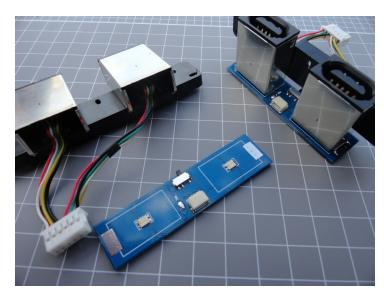
Begin by adding flux to the "dim" pad and make a bead. Next mount the ports on top of the modules and temperately hold them in place with "Blu-Tack". With the soldering iron set to 420°C, add flux and a reasonable amount of solder to the large rectangular grounding pads. Apply some downward pressure while at the same time running the iron up and down the pad until there's a good join between the module and the controller port shielding.
