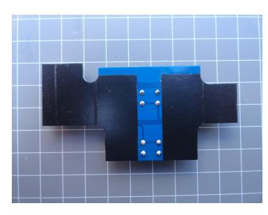
Here's a quick example using typical electrical tape, as you can see on the original there needs to be spaces in the corners for the tabs on the faceplate. Duct tape could over the PCB with a single piece then cut around it with a hobby knife.
