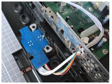
Next insert the XeniumRGB front panel into the faceplate and route the two cable through the hole as shown in the image.
