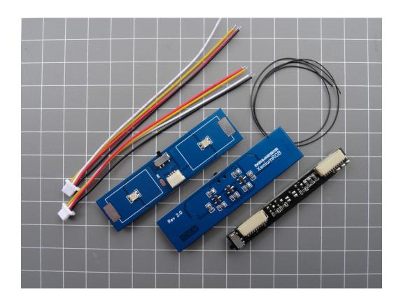
The Xenium RGB Controller Ports are a modified version of the Original Xenium LED module. Which now has dual RGB LED's with a new profile design that can be directly soldered to the back of the controller ports.
