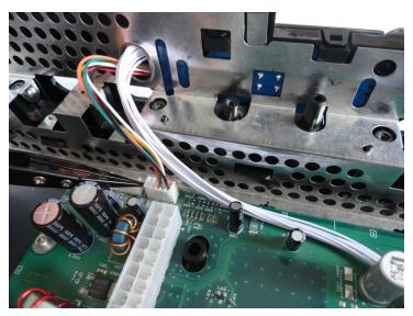
The white 10pin cable is to be connected with the Xenium and the other to the motherboard as shown in the image.
