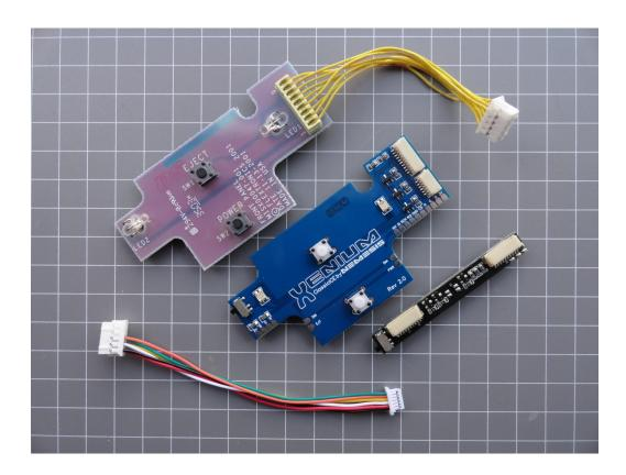
The XeniumRGB front panel is essentially a hybrid of the Original Xbox front panel and the Original Xenium LED module, excuse the missing LED as I used it for my prototype Xenium mod-chip.
