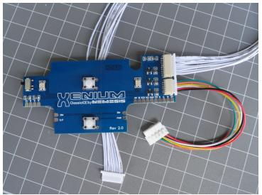
The process for "only" installing the XeniumRGB front panel is solderless.
