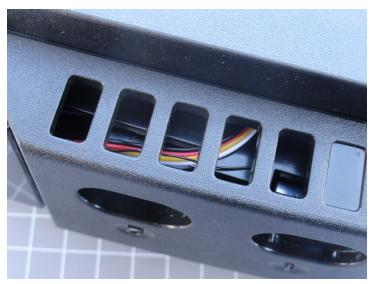
You can loose the remaining slack in the wires by pulling or moving them around from underneath of the faceplate as shown in the image to the left.
