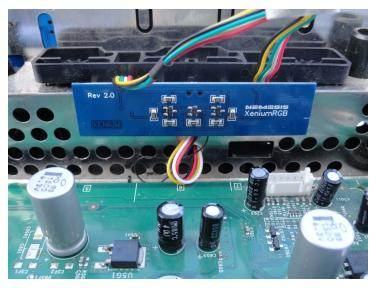
Be careful when inserting the controller ports back into there slots as the wires for the module might get in the way. Try and push them out of the way while the ports and being installed.
