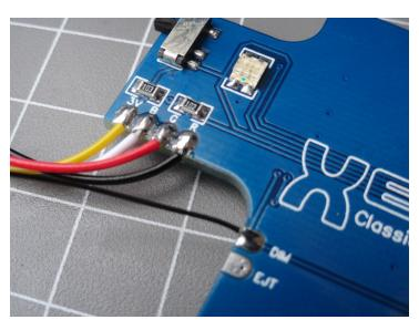
To solder on the wire's first add flux to all the relevant pads and create a nice bead on them. The wires are already tipped so just reheat the pads one at a time and insert the wire tip and remove the soldering iron.
