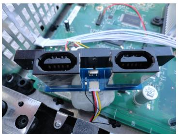
The 4pin cable's are kept short so that there's not too much excess wires for a cleaner install. Attaching the 4pin connector will be a bit tight to work on.
