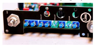
Now it's time to use the Frontpanel for the first time to get the Switches and LEDs in place. Use the spacers and bring the Frontpanel in place with just the Mainboard. You should use the nuts to screw them together. Install the pushbuttons and rearrange the switches on the PCB until they are in the middle of the hole of the Frontpanel. After this process you can solder them in completly. After soldering in all of the Pots and Switches make sure that their leads are also trimmed short.
