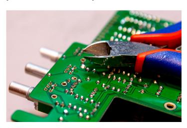
The next step is focusing on the Pot, Grayhill switch and Pushbutton Switches of the Mainboard. Again we will solder just one solder point of each part to bring the Pot/Switch in the right direction and will solder the rest of the Pins later on in the Final Assembly.
