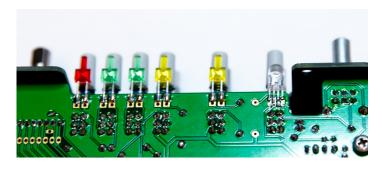
After soldering all LEDs tot the Mainboard unscrew the Frontpanel again. Put the 25mm Spacers on the Mainboard and add the LED-Meter Board. Use the screws to secure the LED-Meter Board. Put the Frontpanel back on again and tighten the Nuts to the bracket. Now we will finally solder the remaining legs of the Pots as they should be perfectly centered now.
