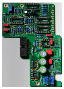
At this point we should clean our board and give the board and us a bigger break. Cleaning boards can be done with alcohol/water/your preferred method. But don't clean the Board after Trimpots, Switches and Pots are installed. Trimpots, Switches, Potentiometers don't like cleaning and that can lead to problems with electrical contact.
