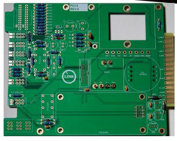
Continue on the LED Meter Board and add all Sockets. Normally we solder first one pin in and trim all of the other Pins as short as possible and continue after that with soldering all other pins on that
