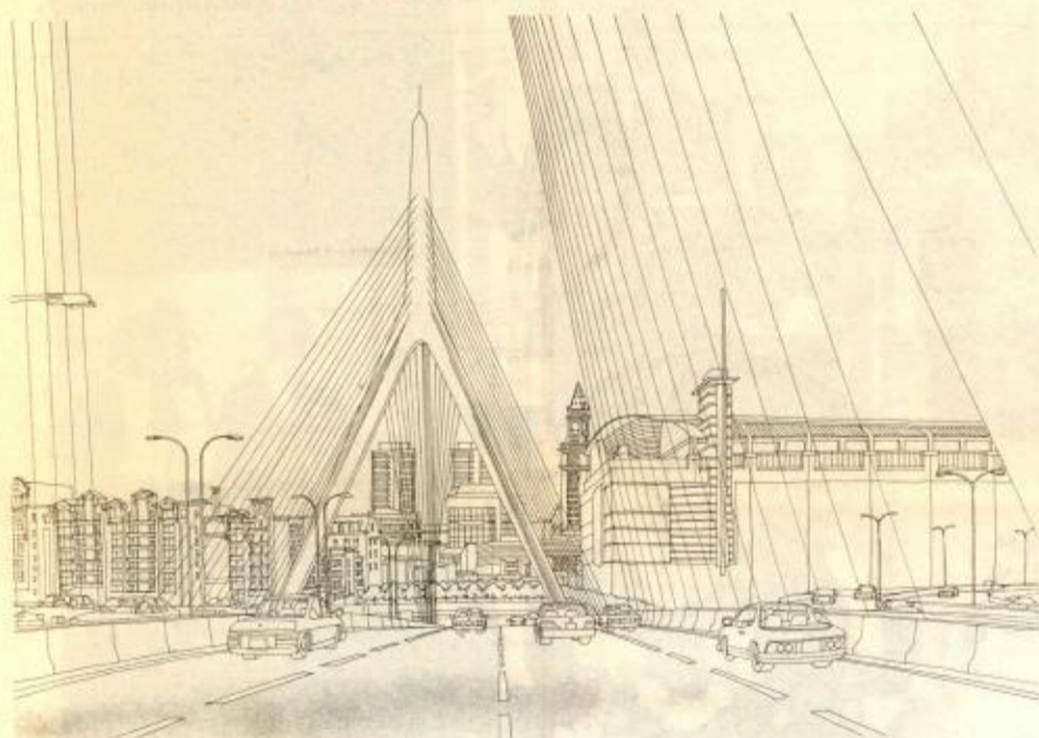
THE CHARLES RIVER CROSSING bridge will serve as the landmark northern gateway to downtown Boston. The cable-stayed bridge pictured here will carry 10 lanes of I-93 traffic. A second, smaller bridge will carry four lanes of traffic between Storrow Drive/Leverett Circle and I-93/Route 1 north.
