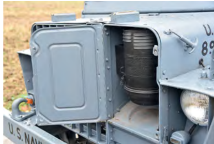
The air filter could be easily accessed and checked daily from the compartment to the right of the grille
