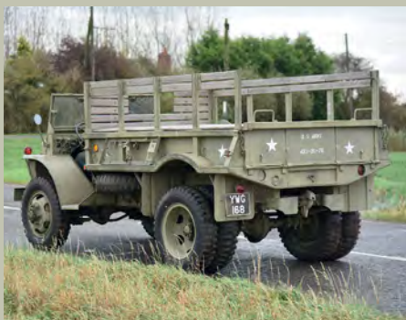
BELOW LEFT: Rugged and ready, easy to visualise on the Ledo Road; note the pull-out tool box above the tow hitch
