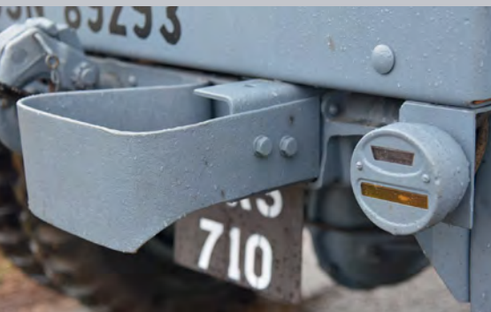
Bumperette and retro-looking, new indicator lights within standard US Guide lamps
