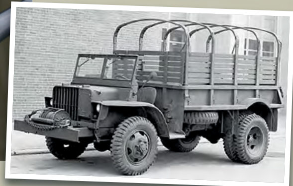
BELOW: The front mounted winch was a common accessory on this truck, either a Garwood or a Braden MU-6; both were well-respected
