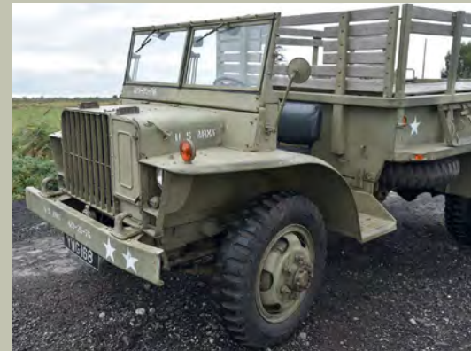
On the cargo truck the spare wheel is stored on the underside of the rear bed, in the bomb truck versions it is positioned on the side of the vehicle
