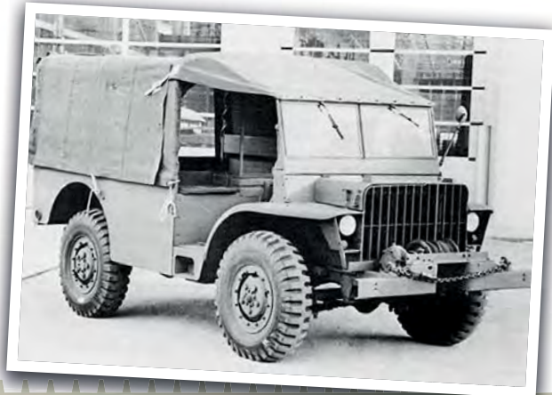
BELOW INSET: Note the single rear set up in this model, only seen on the GTBS version, before reverting to the dual wheel set up in the GTBC
