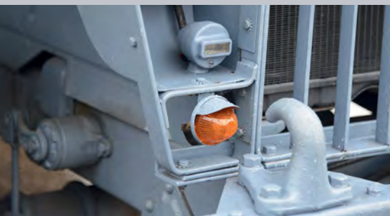
Indicators are the only things not originally on this vehicle. They were sympathetically added later to appease the MOT tester and render it road-legal
