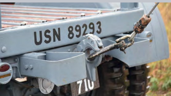
GTB Trucks were designed to pull trailers too, in bomb service, loaded with live bombs destined for aerial bombardment
