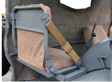
The minimalistic passenger seat offers little comfort, unusually it faces the driver's position and folds away when not in use
