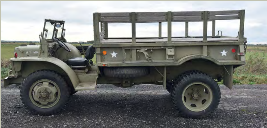
The Cargo truck variant had benches for troops and could be enclosed for shelter with a canvas hood
