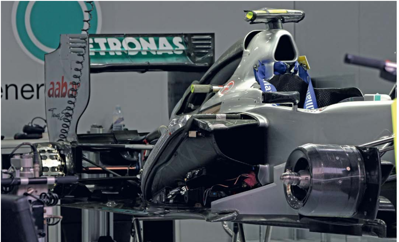
The rear end of the Mercedes W03 has been heavily updated with a switch from an aluminium gearbox case to a lighter carbon fibre design
