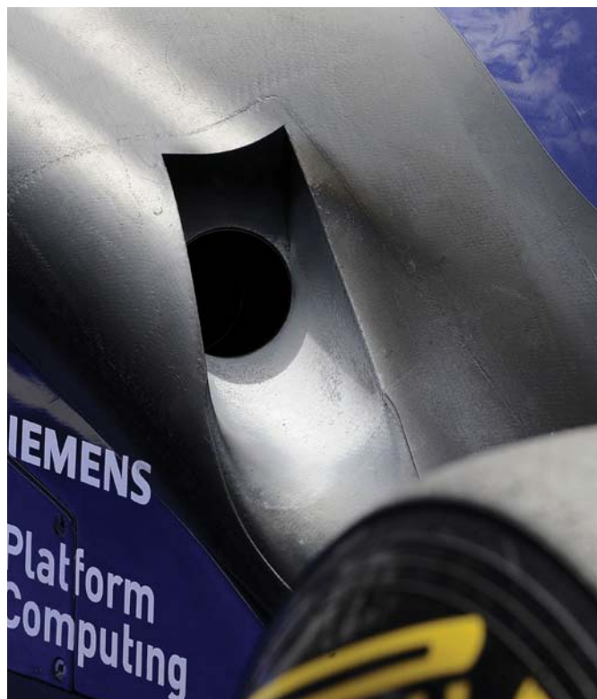
Hot blown floors are outlawed in F1 but attempts to utilise cold blowing continue, as seen here on the Red Bull RB8
