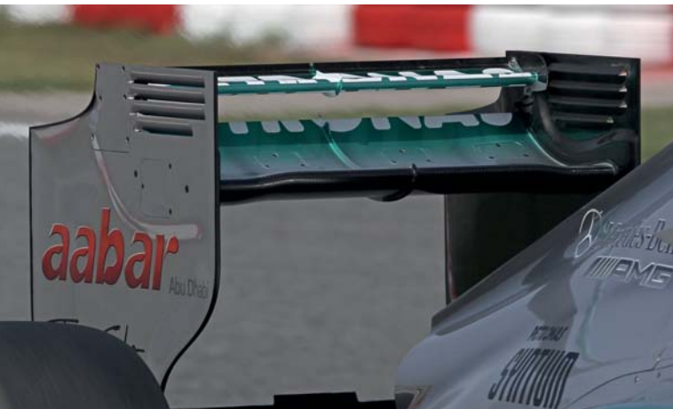
With the DRS open, a small duct is exposed on the rear wing endplate which draws air into two tubes running forward through the car
