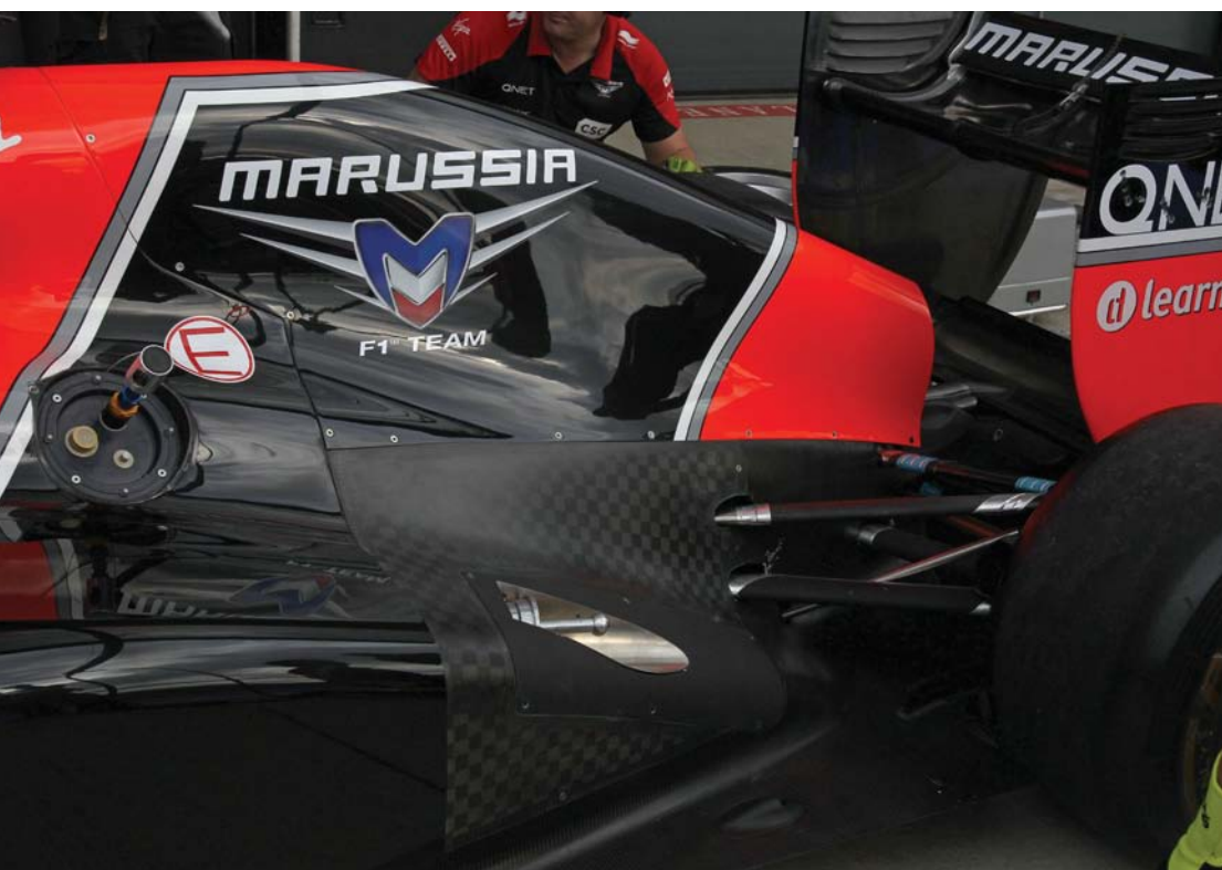
The MR01 started the season with a conventional exhaust exit but was later fitted with a Red Bull style solution
