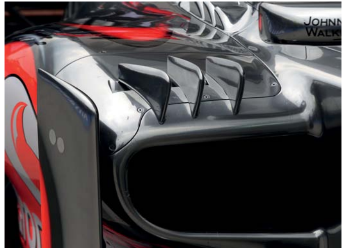
Sidepod wings first trialed by Sauber and then Red Bull appeared on the McLaren after the summer break, taking the place of small turning vanes
