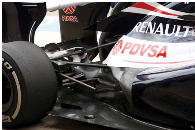
The very low gearbox height is carried over from the 2011 car, as is the clean air flows to the rear end
