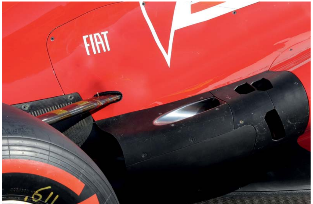
Ferrari circumvented regulations, only allowing a single opening in the bodywork by linking many additional slots and ducts together with tiny cracks. The collection of holes are a single hole in the eyes of the regulations
