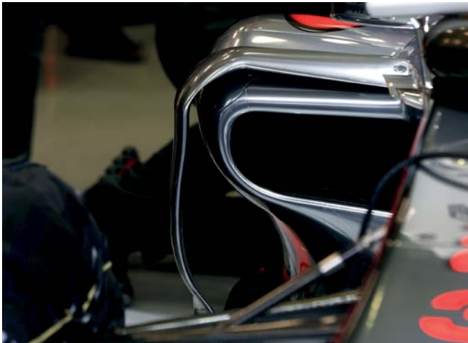
Sidepod wings first trialed by Sauber and then Red Bull appeared on the McLaren after the summer break, taking the place of small turning vanes
