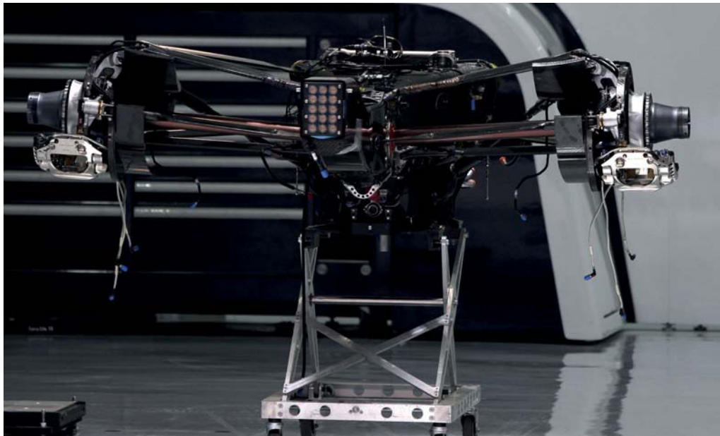
Failures in McLaren's in-house carbon fibre gearbox (also supplied to Force India) have cost the team some points
