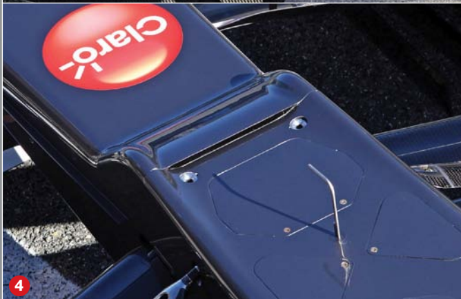
1. Red Bull's 'driver cooling duct' has attracted much discussion 2. McLaren's exhaust exits sit a long way outboard of the chassis and on the limit of the regulatory box. Some have already questioned the legality of the design 3. Ferrari has experimented with many variations of its exhaust in an attempt to re-capture some of the lost downforce 4. Sauber's nose duct faces the opposite direction to the one on the Red Bull
