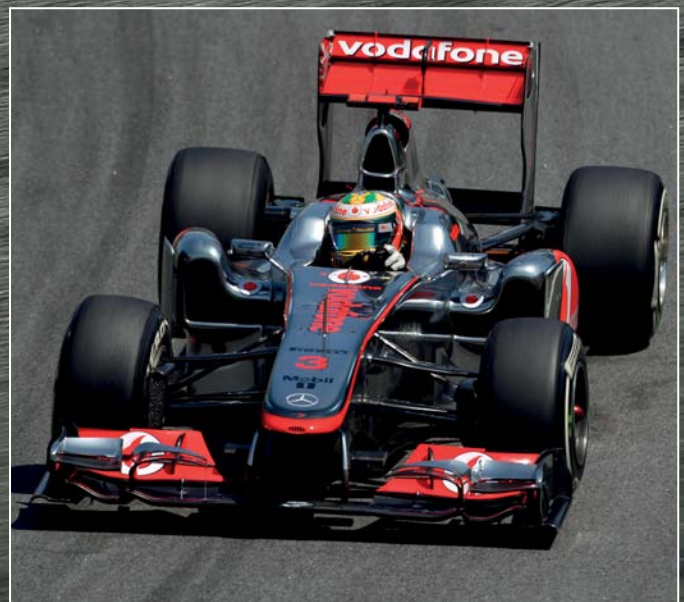
The 2011 MP4-26 featured a distinctive U-shaped sidepod concept, but late changes to the exhaust regulations saw McLaren abandon it. Overall the MP4-26 was a strong basis for the MP4-27
