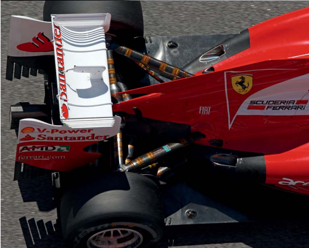
The F2012, unusually, featured pull rod suspension all round, principally for aerodynamic reasons. Whilst the layout is not as good from a suspension design perspective as a push rod layout at the front, the beneficial impact on the air flow outweighs that.
