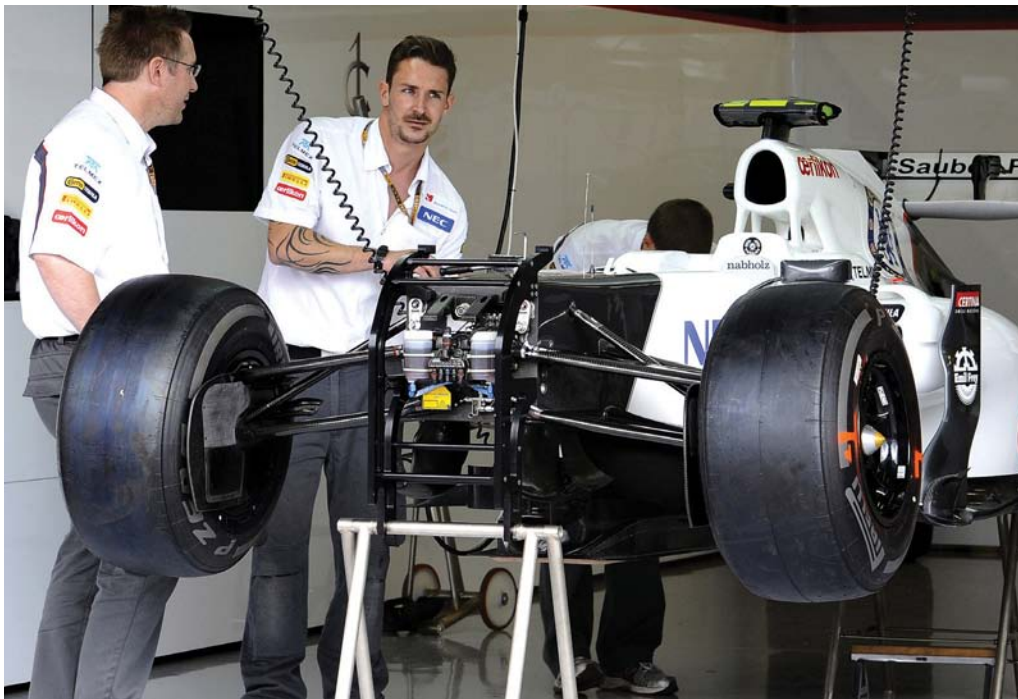
Front suspension was re-designed from the 2011 car but retains the enviable characteristic of being kind on tyres
