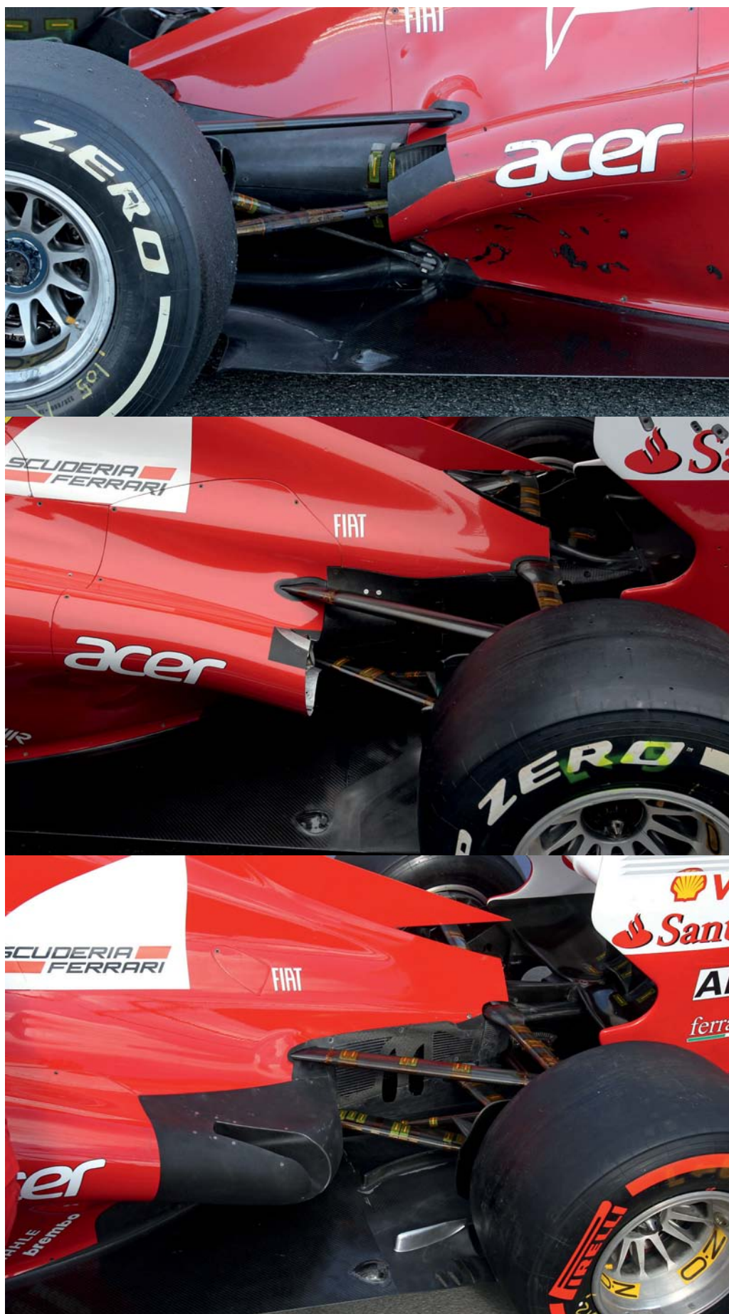
Ferrari struggled with its exhaust design throughout the year. In early versions (top and middle) the aim of effectively generating a blown diffuser was not really achieved. The team did not fully understand why its designs were not working until later in the year when it found issues with its wind tunnel. Sessions in the TMG wind tunnel resulted in a more effective layout used in the final races (bottom)
