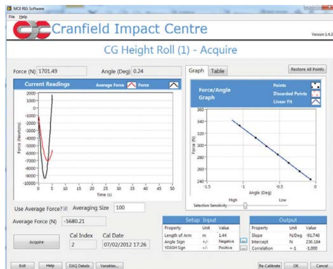
A screen grab of the rig's output when pitch measurement is being taken (left) and with the rig set up to find the c of g height and the car being oscillated in roll (right)
