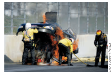
(TOP) Funny Cars are front-engine for sound reasons. (ABOVE) That can be disconcerting when they go bang, but driver protection includes titanium/composite shields.
