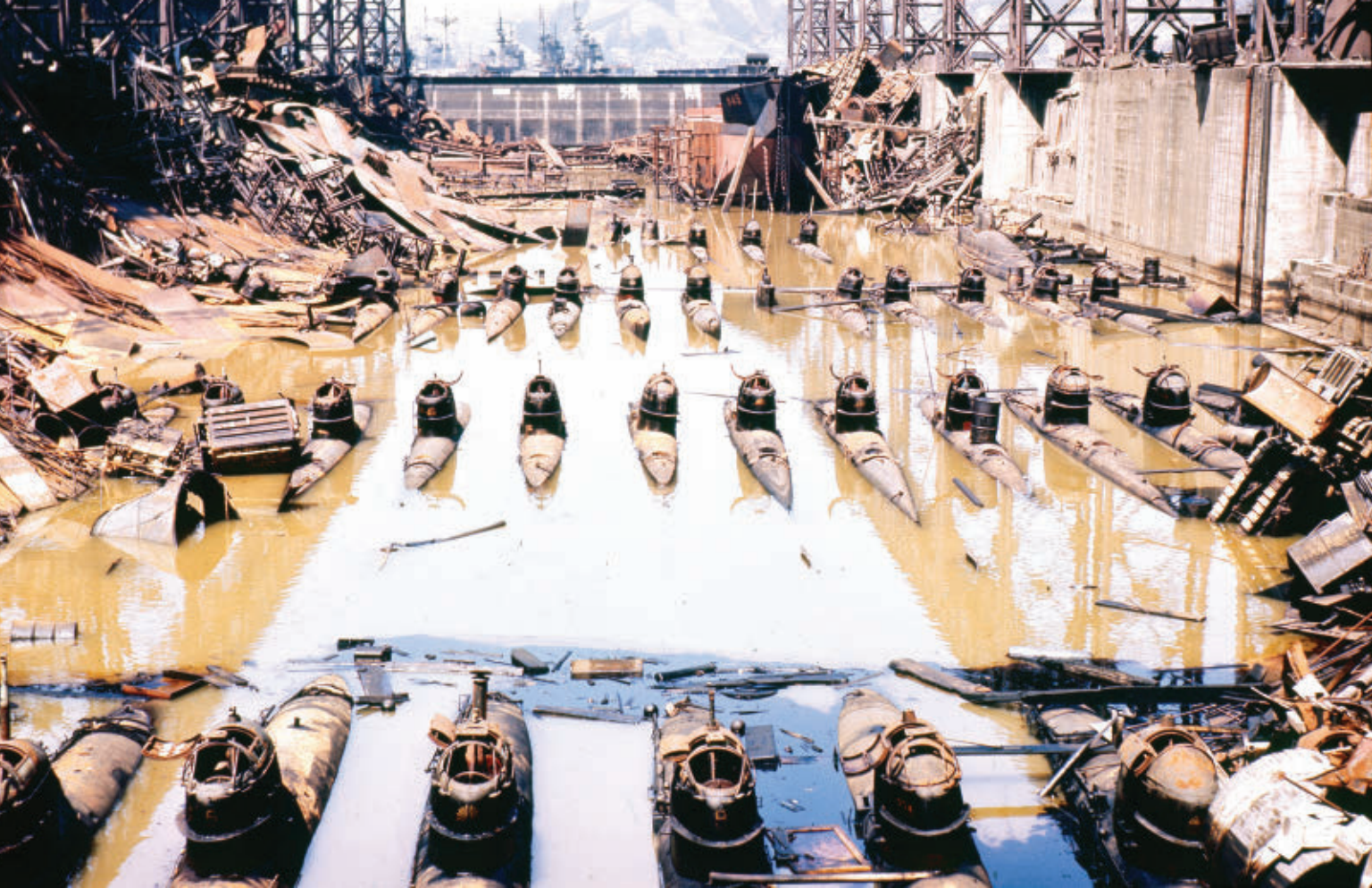
Midget submarines initiated war with the U.S. and were ultimately intended as a last defensive force to protect the Japanese homeland. Seen here were near 80 Type D Koryu subs found in a drydock in Kure in October, 1945. With a crew of up to five and a radius of 1,000 miles these Special Attack Unit craft could have inflicted catastrophic damage to any Allied landing fleet. (Photo courtesy of Stan Plet)
