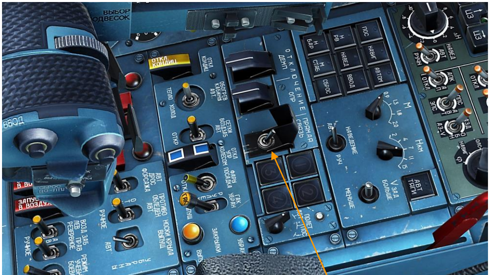
Figure 44: Direct control switch
