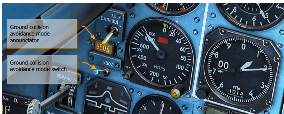
Figure 49: Ground collision avoidance mode annunciator and switch
