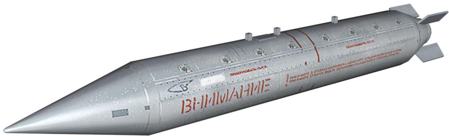
Figure 86: KMGU-2 Sub-munitions Dispenser
