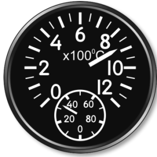
Figure 40: Interstage turbine temperature indicators
