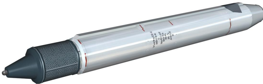
Figure 90: S-25 Unguided Rocket in its Launch Tube
