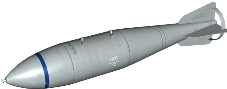
Figure 79: FAB-500 High-Explosive Bomb
