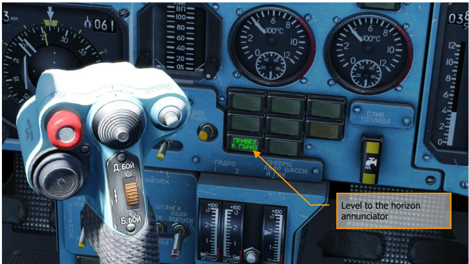
Figure 48: "ПРИВЕД К ГОРИЗ" (Level to the horizon) annunciator
