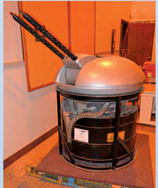
Right: The revolutionary General Electric Central Fire Control system on the B-29 directed four remotely controlled turrets each armed with two .50 Browning M2 machine guns. The turrets on Doc are fully functional, albeit it with deactivated weapons.
