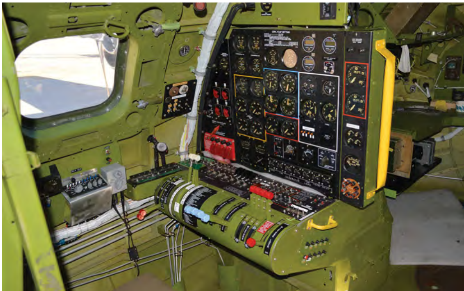
Below: The flight engineer's station on Doc .
