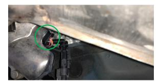
10.) Fasten the cable to the electrical wiring harness in the bumper, e.g. with cable ties. Make sure that the connection line on the servomotor of the exhaust flap has enough room to move and is not under tension.
