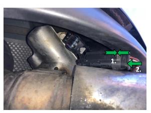
9.) Then connect the plug of the control unit to the servomotor of the exhaust flap until it snaps into place. Push the gray lock in the direction of the servomotor so that the plug can no longer come loose.
