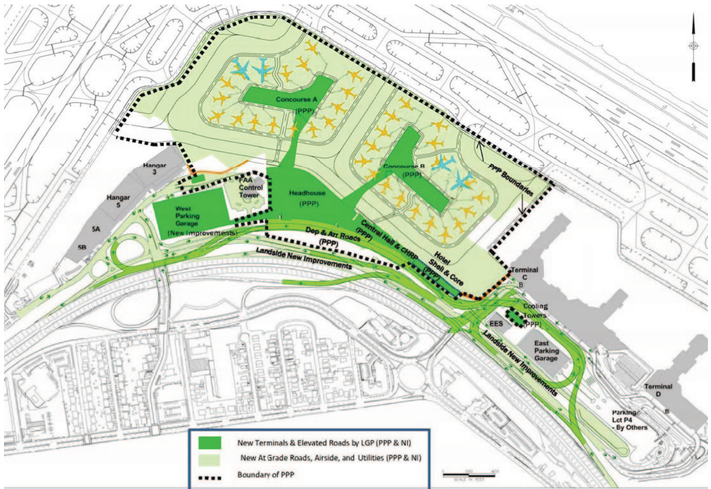
Figure 9.2: Final Terminal Layout
