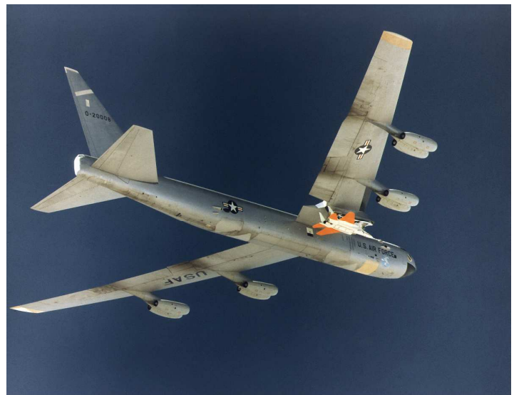
Dryden Flight Research Center ECN-3804 Photographed 1973 F-15 Remotely Piloted Research Vehicle mounted under the wing of NASA's B-52. NASA photo
