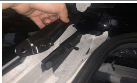
4. Remove the original vehicle bracket and install our body bracket ("L" left "R" right)
