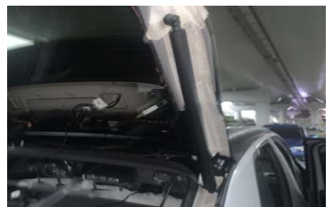
6. Install our electric pole ("L" left "R" right)
