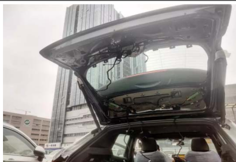
3. Remove the tailgate trim panel
