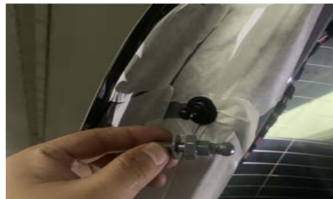
7. Remove the original ball head of the rear door and install our ball head(same left and right)
