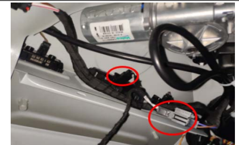
10. Unplug the button line of the original car tailgate and dock with our lin
