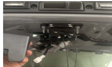
8. Remove the original lock and install our upper lock
