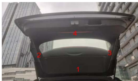
2. Remove the tailgate trim panel
