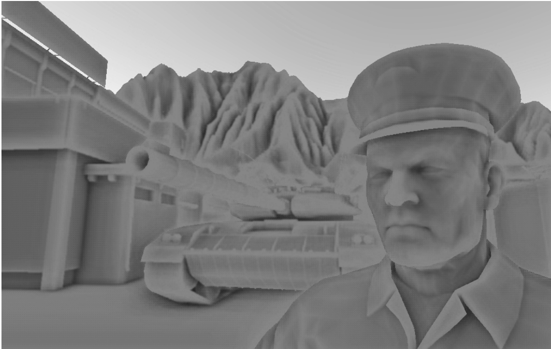
Figure 3.8: This image shows the effect of ambient occlusion on a video game scene. Image courtesy of Mittring [18]
