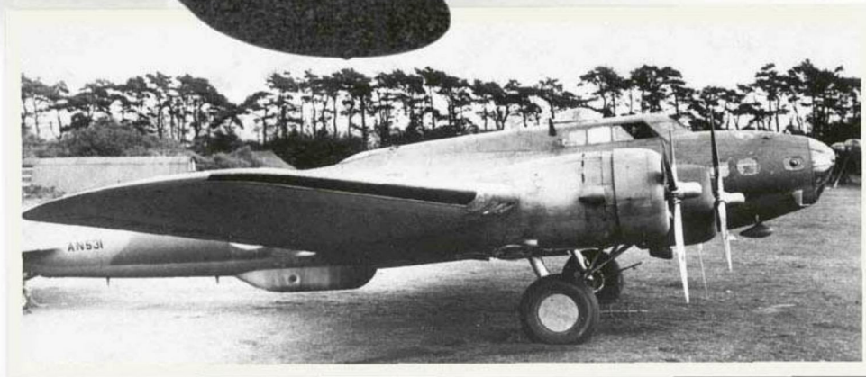
The longest serving Fortress I with the RAF was AN531, which was not retired until January 17, 1945. Note one of the many distinctive features of the early Fortress under the rear fuselage. This was a ventral gun blister contained within a metal housing nicknamed the "bathtub turret", which would be replaced by the ball turret in later variants of the B-17.
