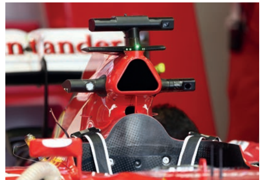
The roll hoop and engine intake, coupled with the mandatory camera mountings
