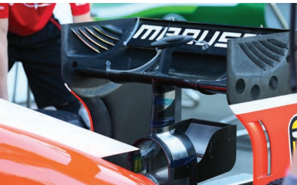
Close-up view of the Y-lon rear wing support
