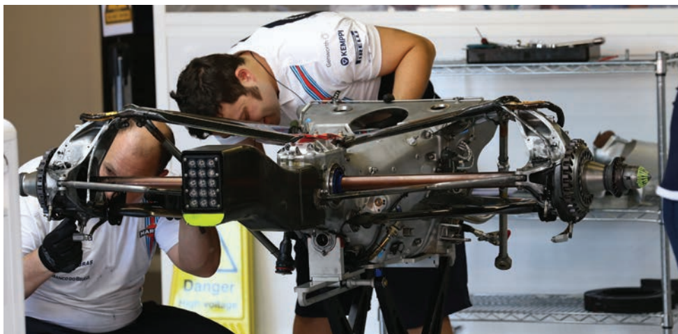
The exposed rear end of the Williams FW36 – the metal transmission casing evident as is the composite rear crash structure. Note the neat rear upright designs
