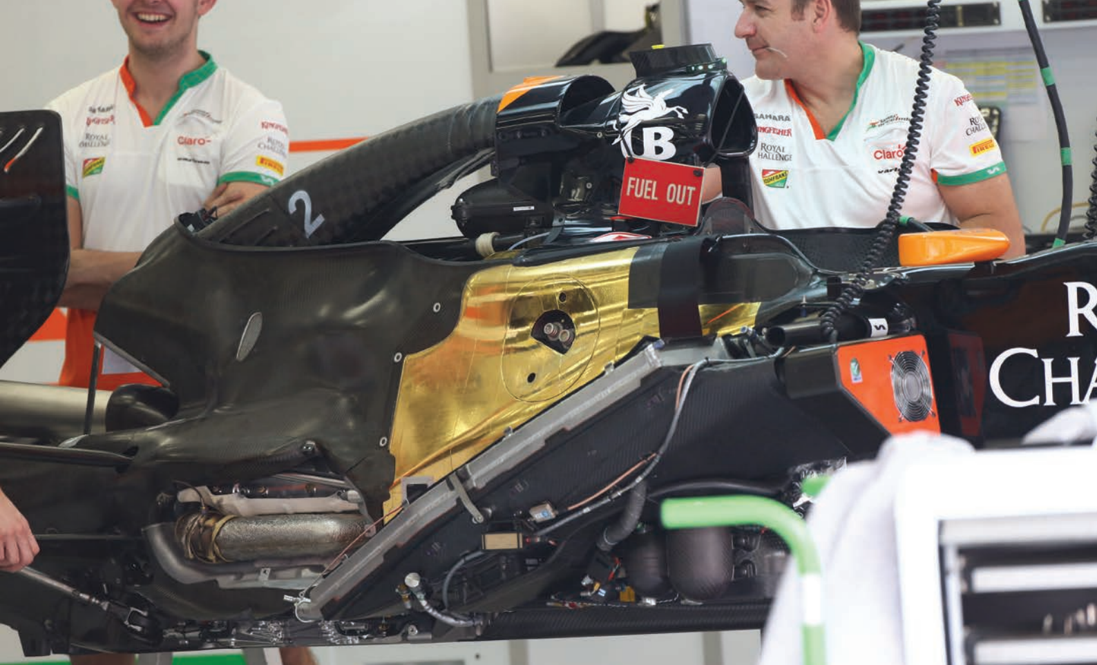
The team cars look almost identical and meet weight regulations, but one chassis is built on a lighter carbon monocoque
