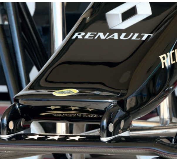
An experimental 2015 nose signals next season's replacement for the Lotus twin-tusk nose design
