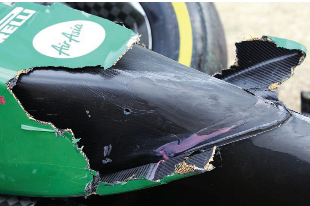
The crash at the Australian Grand Prix damaged the CT05's vanity panel, exposing the true shape of its nose structure
