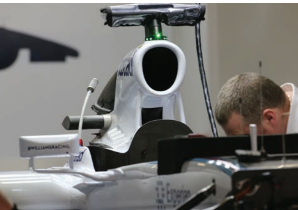
Roll hoop of the Williams FW36 with cooling slots evident. Note the engine air intake with its hybrid safety light
