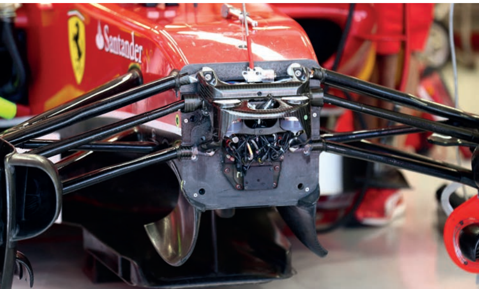
The bulkhead showing inboard wishbone mounting and controversial pullrod front suspension layout
