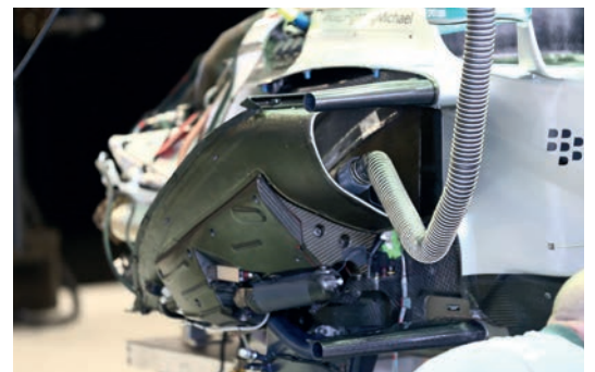
Mercedes' very clean look extends to the side pod – the space beneath the duct devoid of the usual clutter of hydraulics
