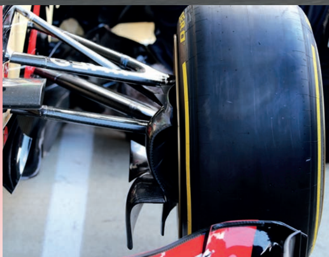
Wheel and tyre sizes have been fixed for a long time in Formula 1, while fans have become used to the aesthetics of low profile rubber elsewhere. Changes – as flagged by Lotus here – will mean a major rethink in chassis and aero design
