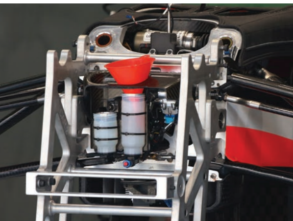
The front bulkhead is machined from billet, unique in current top level racecar construction. Note the spring damper unit between the torsion bar holes
