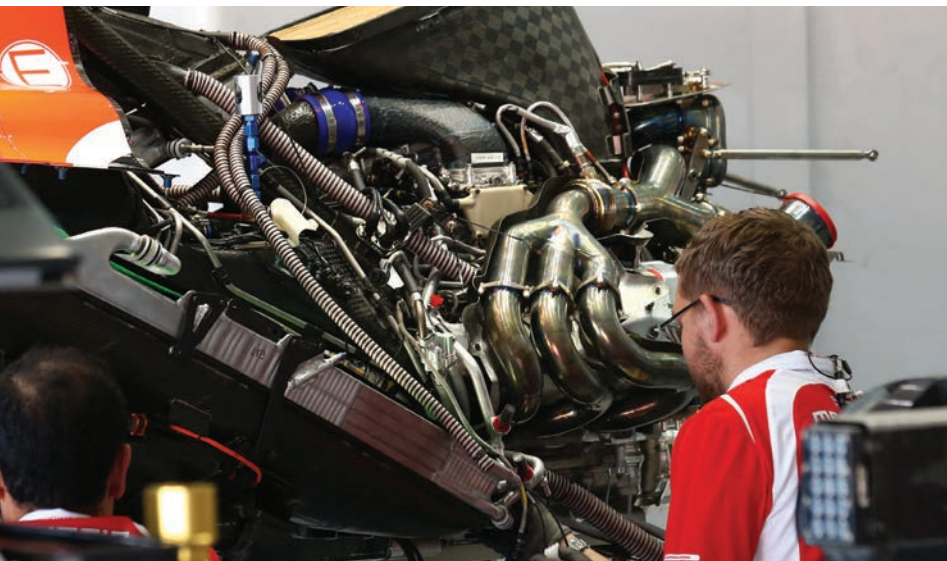
The rear end of the MR03 with heat shielding and transmission removed – many interesting things to see here
