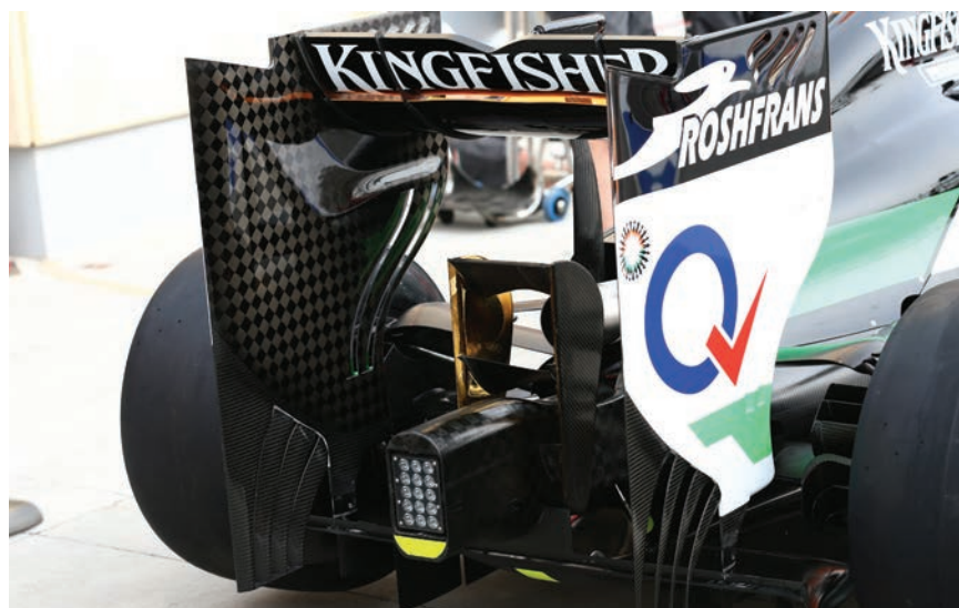
The aero-assisting Coanda exhaust system is outlawed for 2014, with all cars on the grid now restricted to a single central tailpipe
