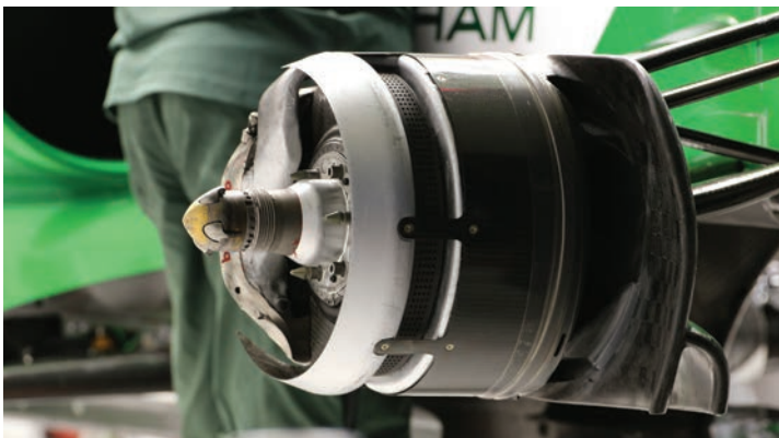
Front brake setup, with some of the aerodynamic elements visible
