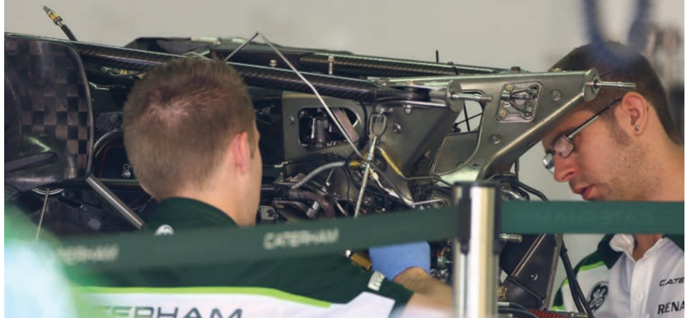
Red Bull developed two transmissions for the 2014 season, one for the RB10 (top) and the other for the Caterham CT05 (above). The forward section of the first iteration of the former is believed to have had to be reworked due to its unfortunate tendency to catch fire, while the latter features a metal forward section which did not suffer from similar issues.
