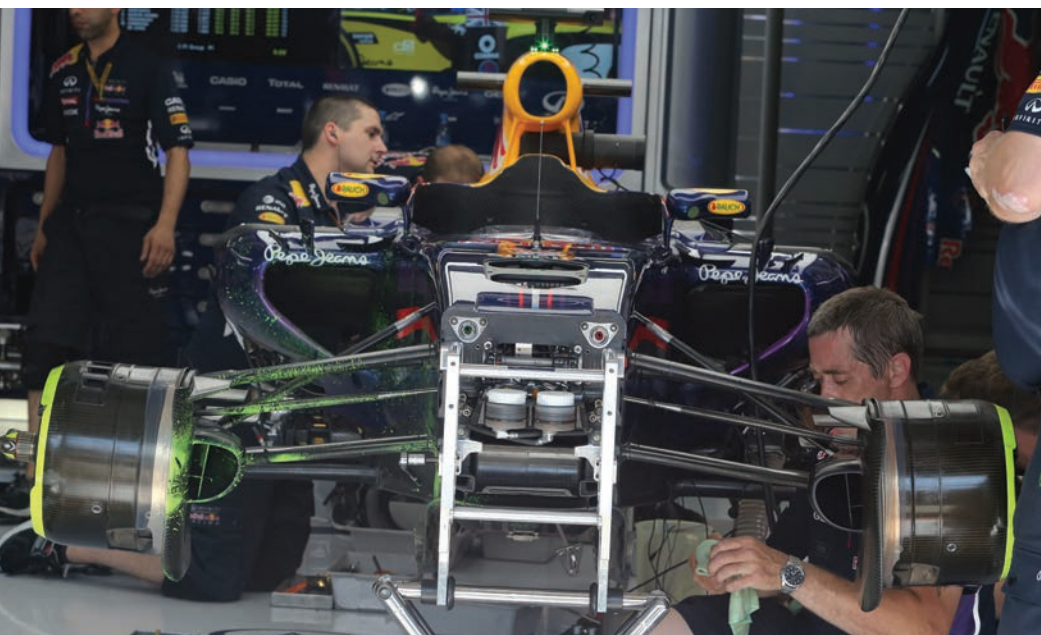
The RB10 retains the long-established Red Bull suspension layout of pull rod-actuated dampers and torsion bars at the rear and pushrod at the front. At the start of the season it featured a front-to-rear interconnection but this was dropped when the legality of such systems was questioned mid-season
