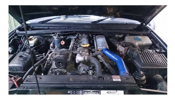
Disconnect all the electrical connections around the head, thermostat, glow plugs etc. Followed by all the hoses, coolant and intercooler etc.
