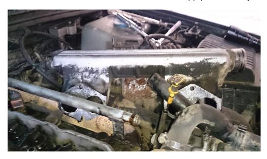
Following this I removed the inlet manifold, this is held on by 2 bolts and 2 nuts then it pulls up and away.
