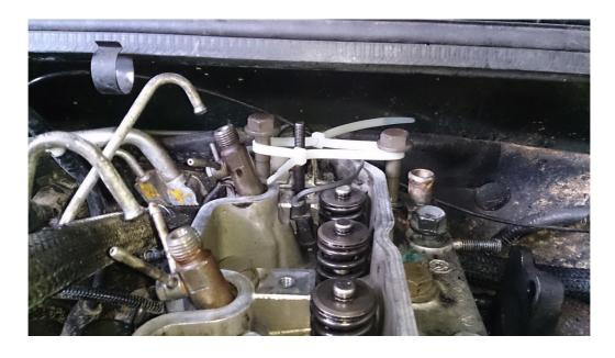
The head has to be torqued to 40nm then 60 degrees followed by another 60 degrees then 30 degrees on the 12mm bolts. A handy tip here is you don't need a dial gauge as each flat on the bolt head is 60 degrees, I used a dob of white paint one each bolt head for each torque setting.
