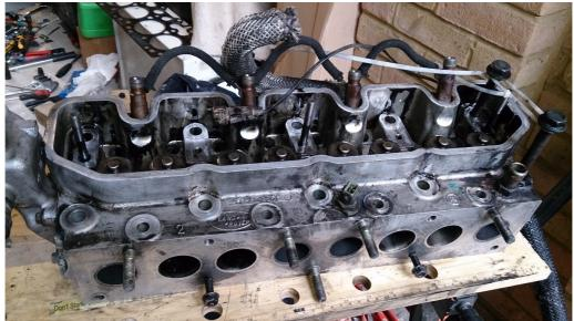
When refitting the head the 2 head bolts nearest the bulkhead have to be inserted before the head is placed on the block, I used cable ties to hold them in place.
