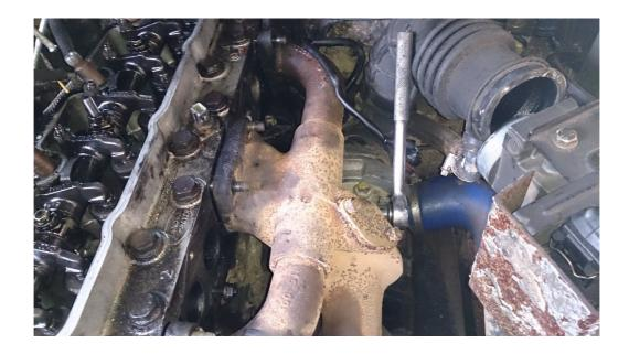
The rocker gear is held by 3 nuts and 2 bolts and lifts off as one piece, then remove the pushrods but keep them in order by putting them in a piece of cardboard.
