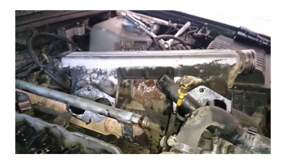
The exhaust manifold simply unbolts except for the centre bottom nut, its seems impossible to get at, this had scratching my head for some time, then I found out you can get a 15mm 3/8" drive socket in beside the turbo as shown below.
