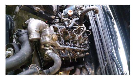
Then it's basically putting it all back in reverse order, with new gaskets where required and resetting the tappets.
