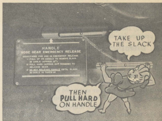
Figure 3-11. Nose Gear Emergency Release Handle (On Radio Operator's Floor)
