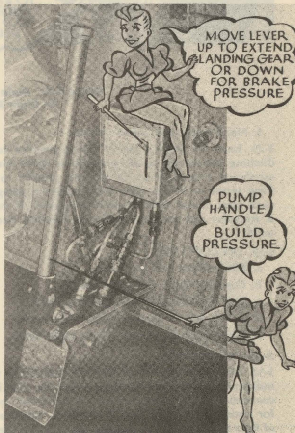
Figure 3-9. Emergency Hydraulic System Controls (On Radio Operator's Floor)
