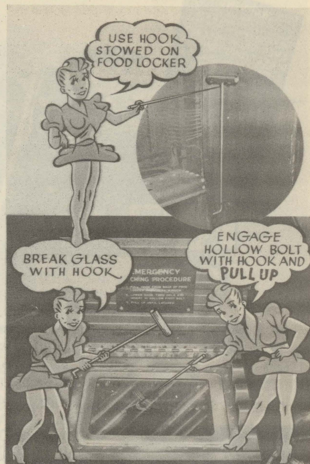
Figure 3-12. Nose Gear Emergency Latching (On Radio Operator's Floor)
