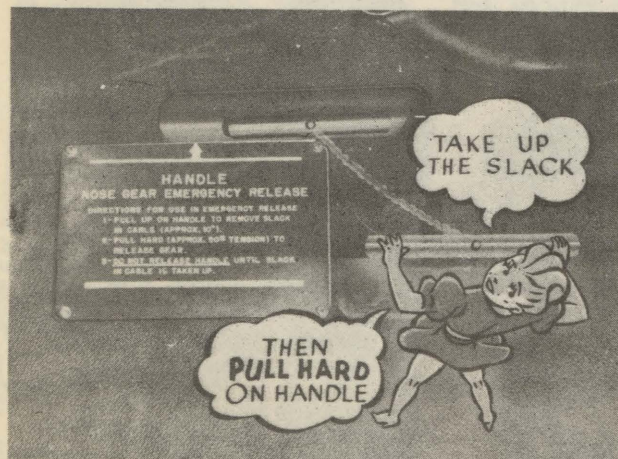
Figure 3-11. Nose Gear Emergency Release (On Radio Operator's Floor)
