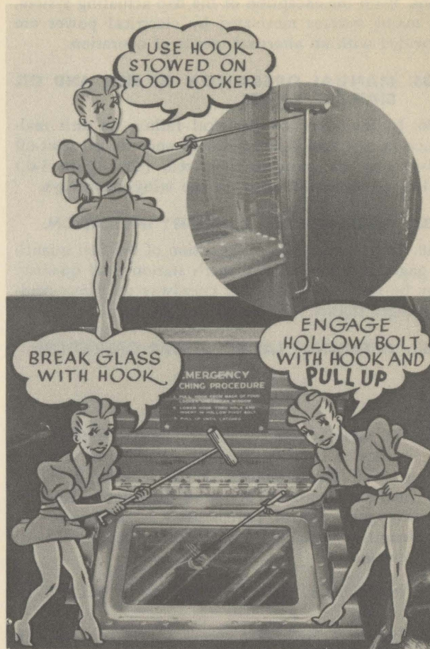
Figure 3-12. Nose Gear Emergency Latching Hook (On Radio Operator's Floor)
