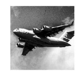
However, when we have a color image, we first need to convert the image to the YUV color format. The Y is the luma, or brightness, and U and V denote the color. After the conversion, we can apply equalizeHist to the image and then convert it back to BGR or RGB:
