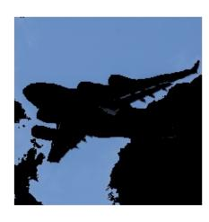
Isolating colors in OpenCV is straightforward. First we convert an image into HSV (hue, saturation, and value). Second, we define a range of values we want
