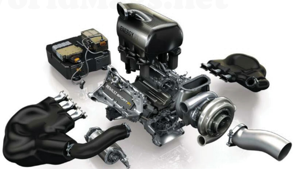
(Above) exploded view of Renault's new F1 power unit; (left) problems for the Red Bull RB10 in testing at Jerez, as Daniel Ricciardo was forced to stop on the circuit, and a fire extinguisher was put on the case
