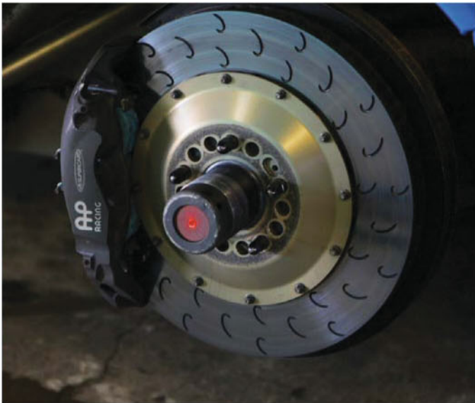
The S60 V8 features AP Racing four piston caliper brakes
