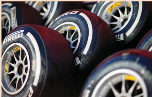
Pirelli also brought a new design of tyre to the Bahrain tests, with 2014 construction and compound. However, these are actually considered to be 'prototypes', as their purpose is to test tyre behaviour without warming blankets, which will be banned from 2015 onwards
