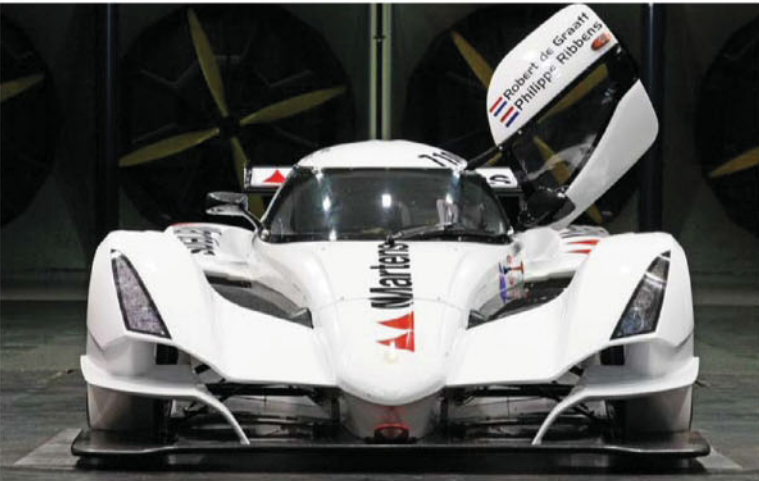
View of the nicely radiused, raised splitter leading edge and integrated devices between the wheel pods and chassis, and between wheel pods and splitter
