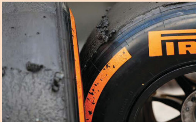
Pirelli also brought a new design of tyre to the Bahrain tests, with 2014 construction and compound. However, these are actually considered to be 'prototypes', as their purpose is to test tyre behaviour without warming blankets, which will be banned from 2015 onwards
