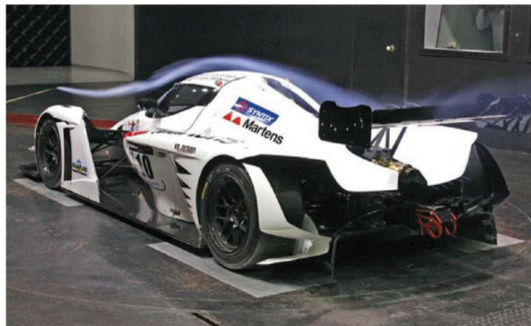
Rear quarter view shows clear areas between the front wheels and the chassis
