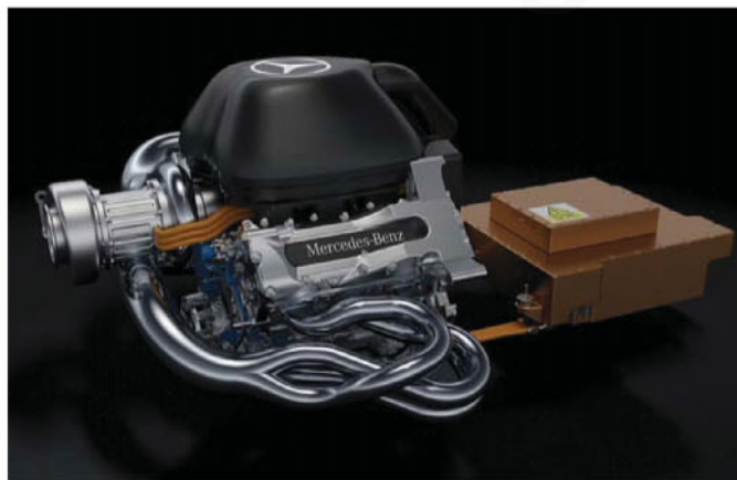
Mercedes AMG Petronas is believed to have gone down an air-water-air route of cooling but offers its customer teams a choice
