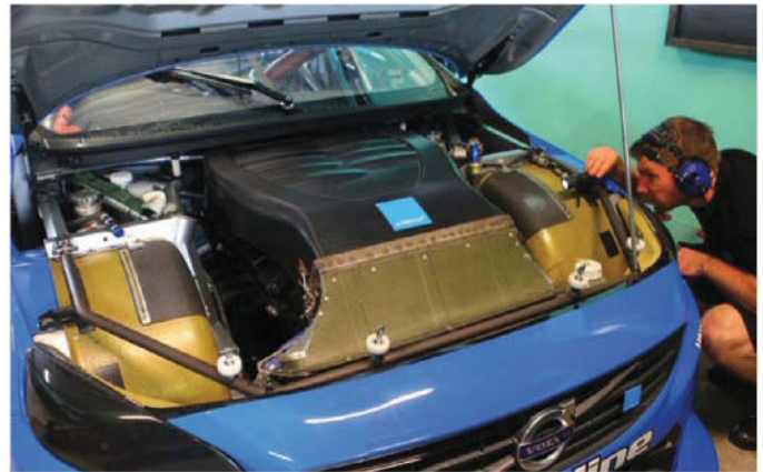
Volvo's Supercars engine programme consists of leftover stocks from the Yamaha-designed B8444S previously seen in S80 and XC90 road cars
