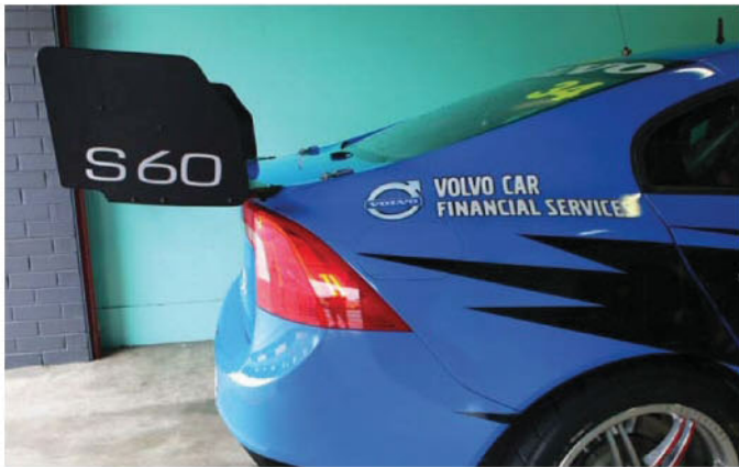
The S60's boot is 150mm shorter than the Commodore, meaning that the rear wing protrudes quite a way off the back of the car
