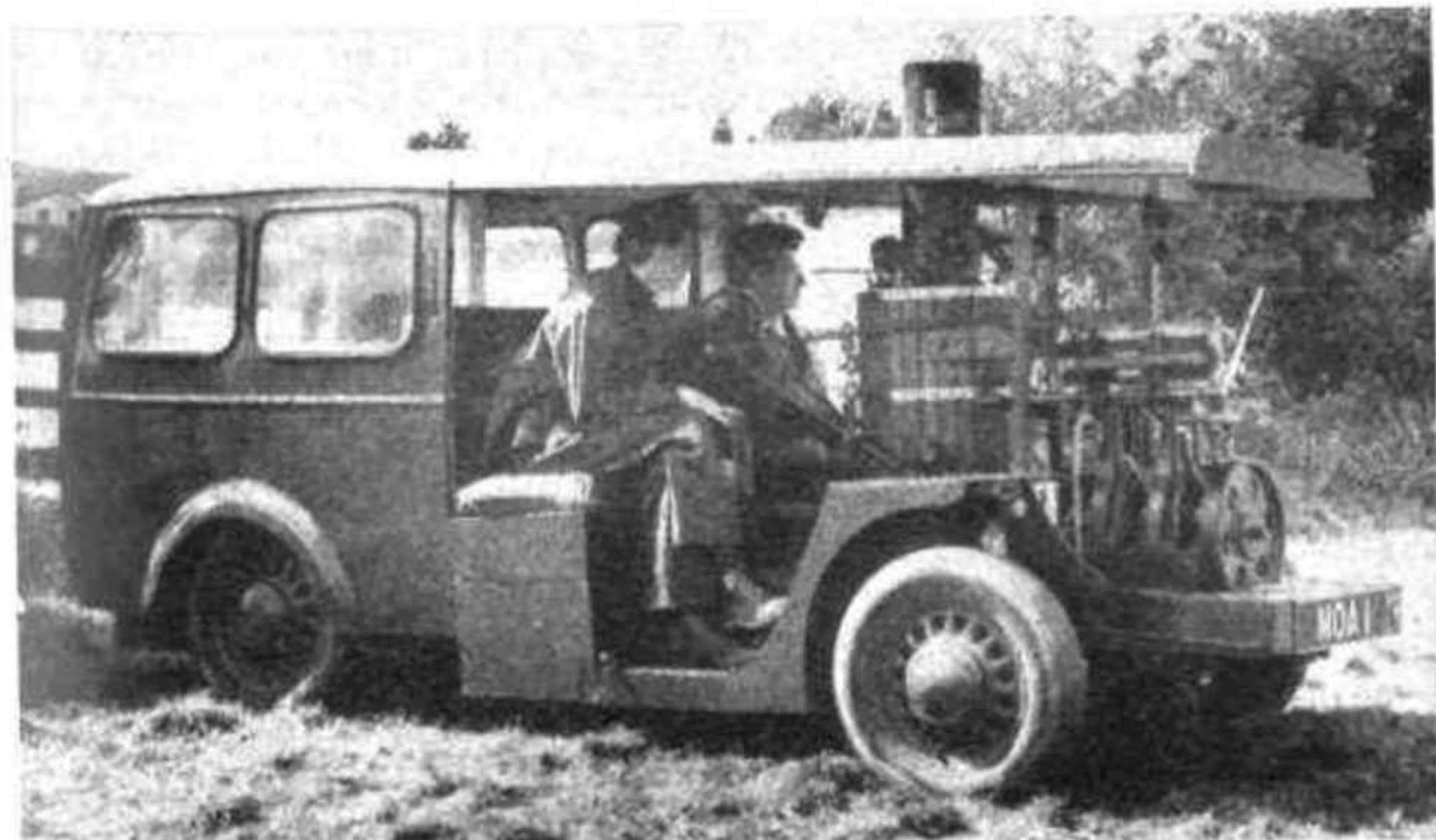
The steam-driven Jowett Bradford, "The Novelty", one of the few home-built steam cars we have encountered which is actually used on the road.
